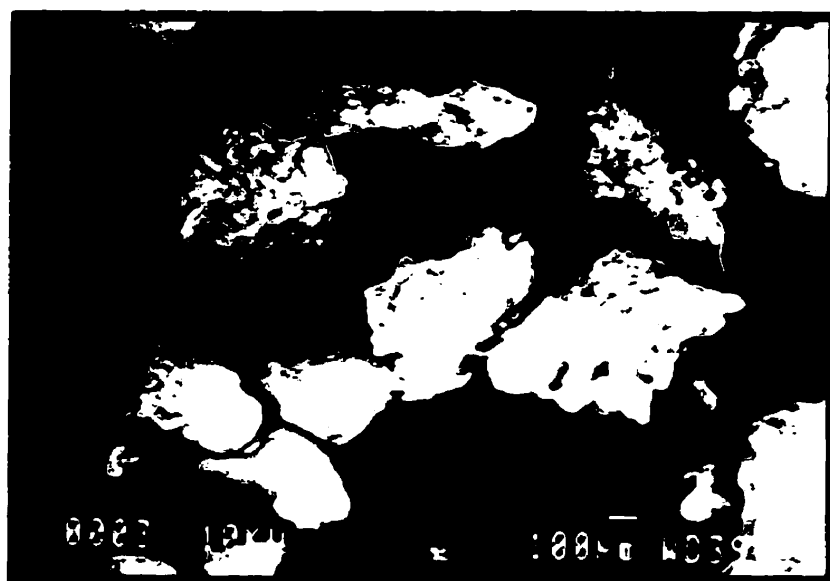
Figure 5.5 Scanning electron micrograph of bottom ash after beneficiation
