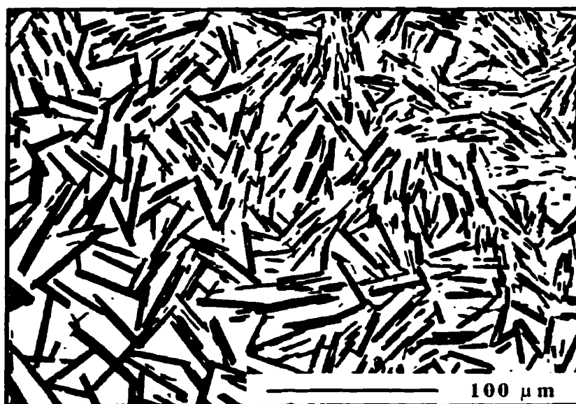
Figure 5.25. Scanning electron micrograph of the surface of the bulk fly ash glass heat treated to 1200° C
