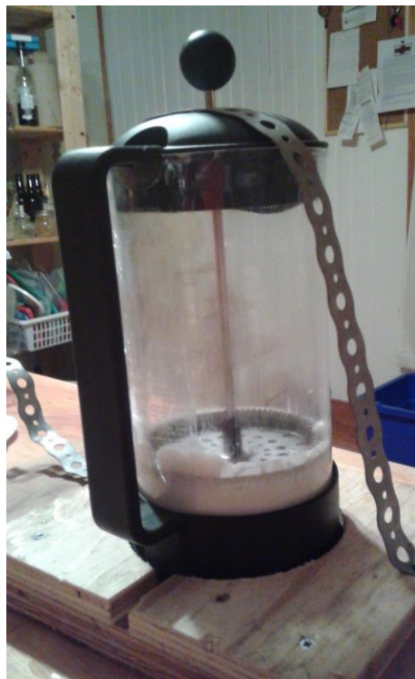
Figure 9: Coffee press apparatus used for testing different mesh materials.
