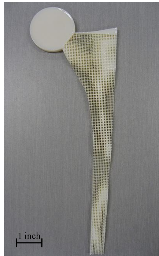
Fig. 9 Polypropylene proof-of-concept of the optimal graded cellular implant (solution B)
