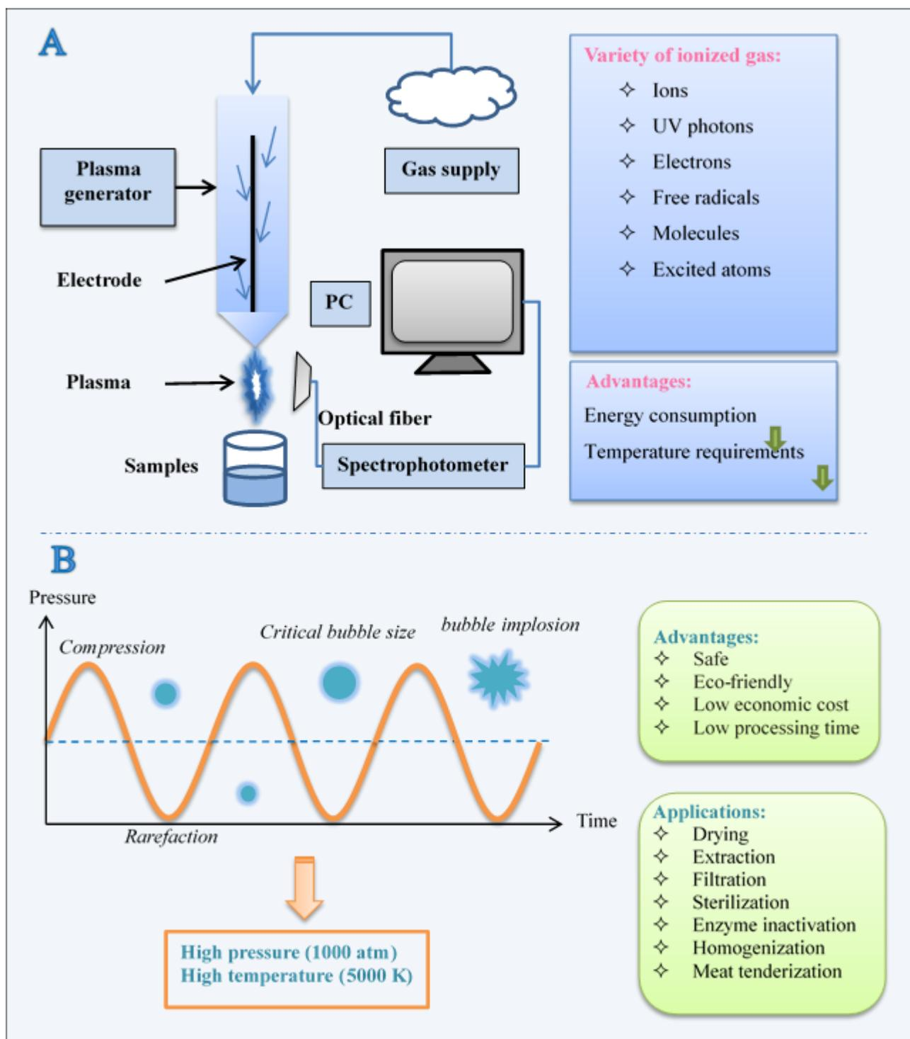
Figure 2.6. (A) Mechanisms and advantages of cold plasma processing system; (B) Mechanisms and applications of ultrasound processing system
