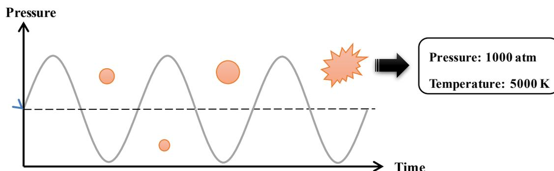
Figure 3.3. Mechanisms of ultrasound assisted extraction principle and cavitation phenomenon
