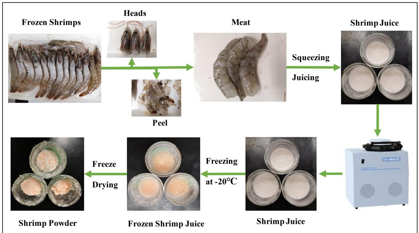
Figure 5.1. Schematic overview of the pretreatment of shrimp samples
