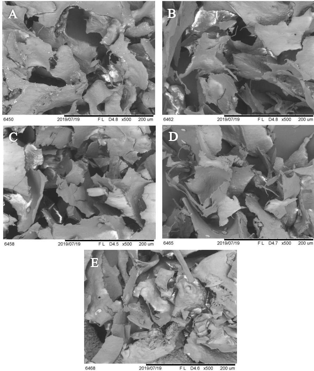
Figure 4.9. SEM photomicrographs of freeze dried shrimps (A) US0 (untreated sample), (B) US-5, (C) US-10, (D) US-15, and (E) US-20 (magnification at 500×)
