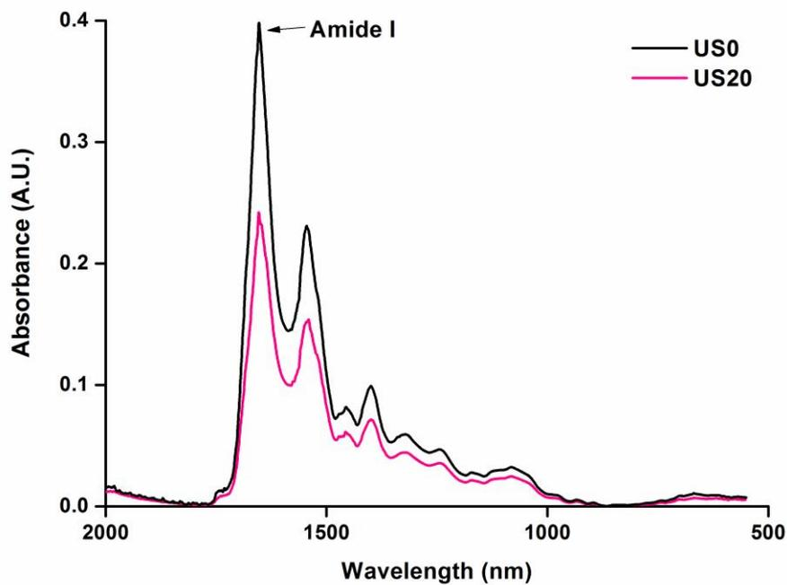
Figure 4.4. FTIR spectrum of shrimp samples with and without ultrasound processing
