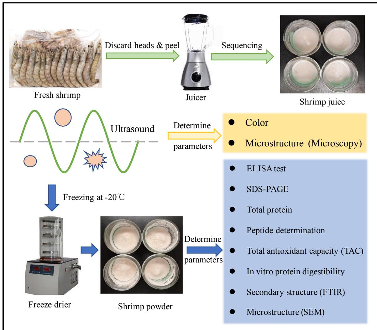
Figure 4.1. The overview experiment scheme including (A) Frozen shrimps, (B) Fresh shrimp juice, (C) Freeze dried shrimp samples
