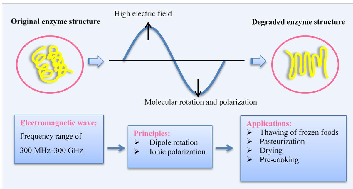
Figure 3.2. Molecular rotation mechanism and applications of microwave heating process
