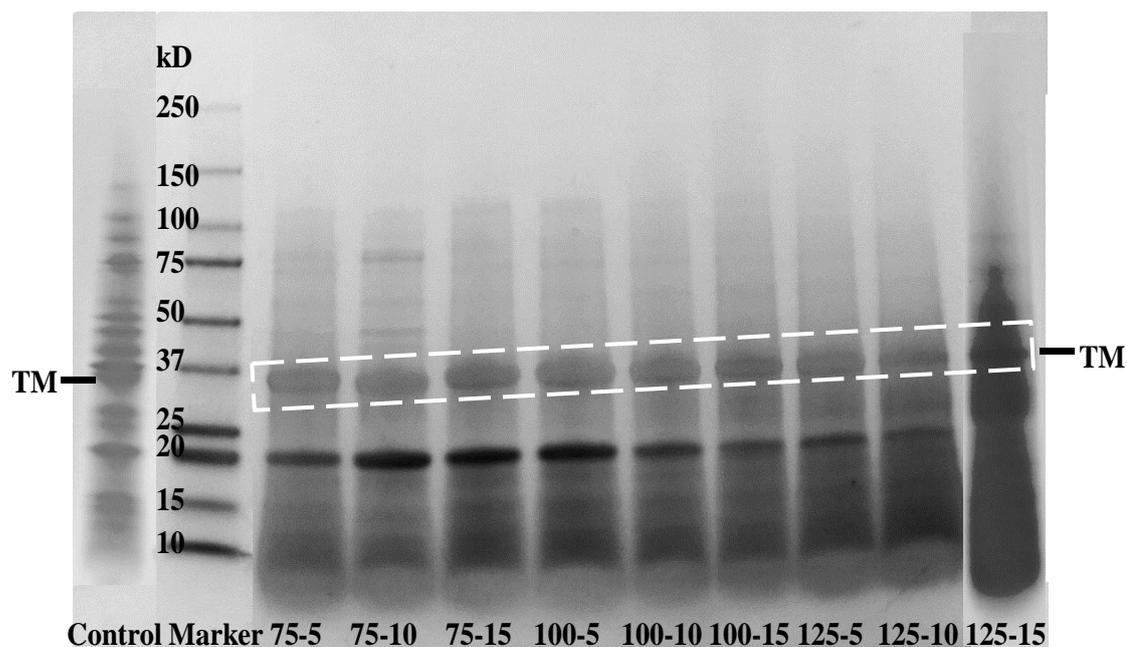
Figure 5.6. SDS-PAGE of microwave treated and untreated shrimp samples
