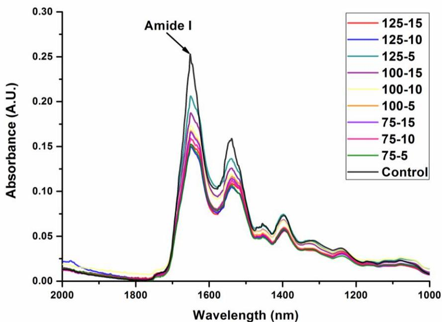
Figure 5.4. FTIR spectrum of raw and microwave processed shrimp samples
