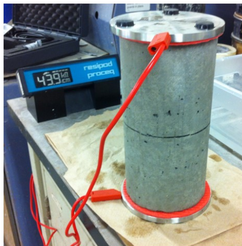
Figure 8: Measuring bulk resistivity
