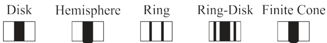
Figure 1.10. Several UMEs geometries including disk, hemispherical, inlaid ring, ring-disk, and finite conical
