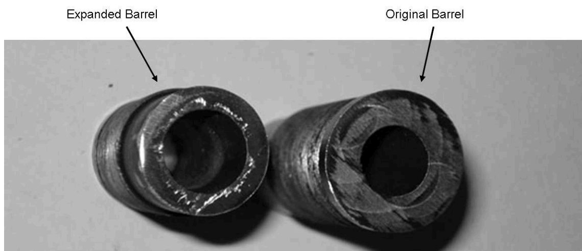
Figure 3-2: Before and after of a barrel expanded by multiple high pressure gun cycles
