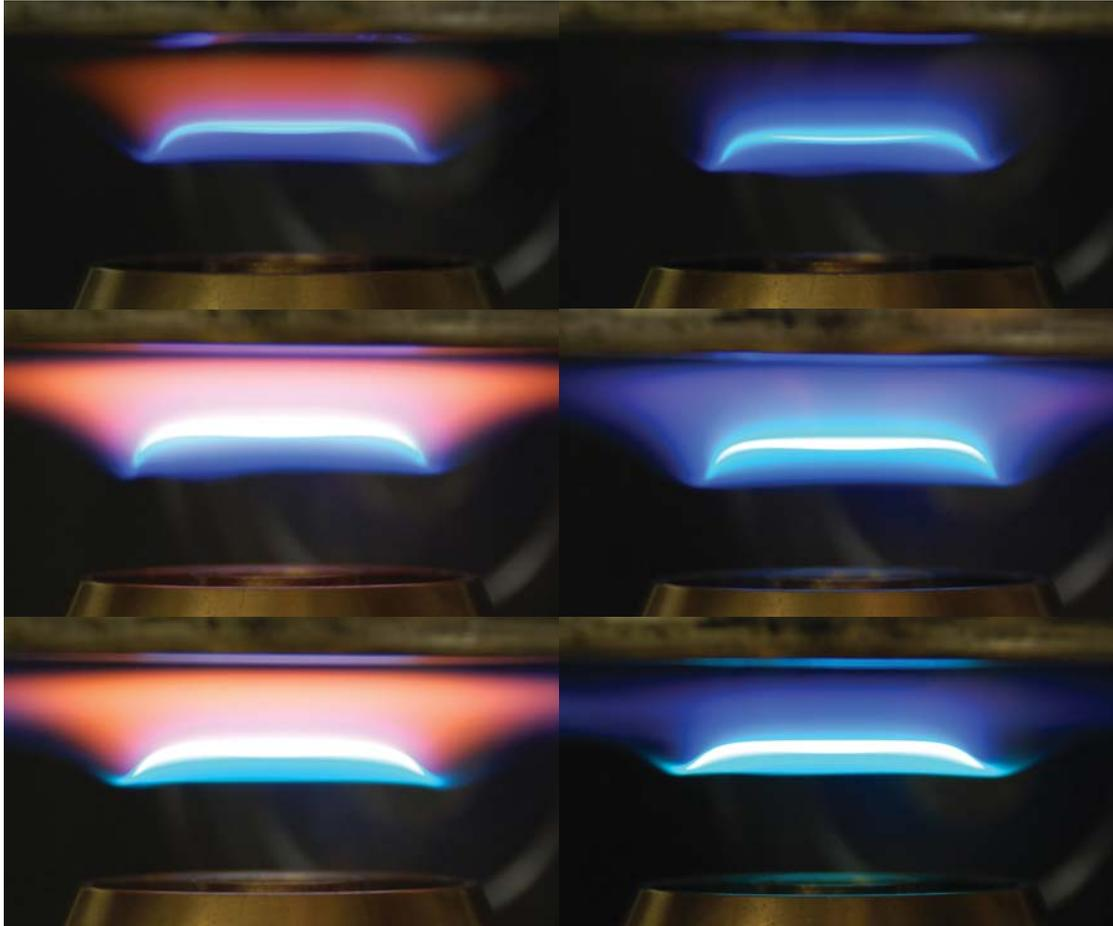
Figure 5-5: Photo of *n*-butanol (left) and *n*-butane (right) stagnation flames:  $\phi=0.8$  (top),  $\phi=1.0$  (middle),  $\phi=1.3$  (bottom)
