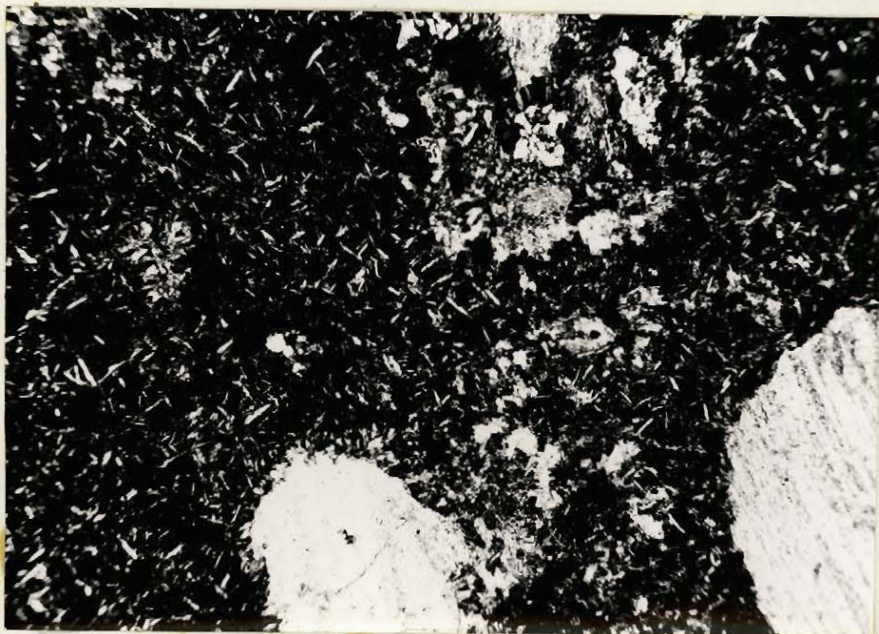
Figure 21. Amygdaloidal basalt, one mile south of Ayers Lake. The Amygdules are calcite. Crossed nicols, X 26.
