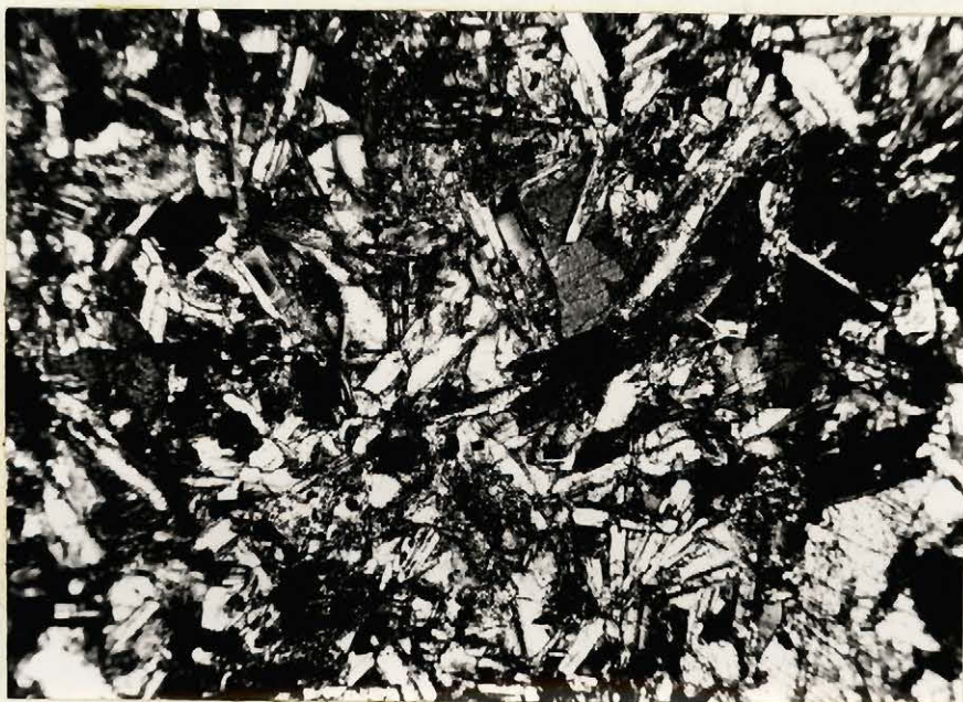
Figure 23. Diabase sill in pre-Silurian sediments, exposed on the road about 2 miles east of East Newbridge. Crossed nicols, magnification X 26.
