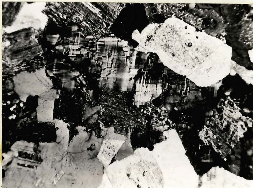
Figure 22. Biotite granite; in railway cut about \frac{1}{2} mile north of Barton. Crossed nicols, magnification X 26.
