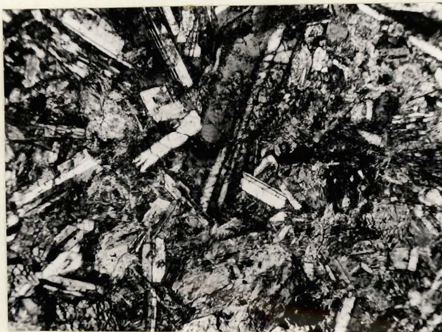
Figure 25. Diorite, one mile southwest of Colter Lake. Feldspar are largely twinned, and appear white or grey in the figure, the remainder is highly altered ferromagnesian. Crossed nicols, X 26.
