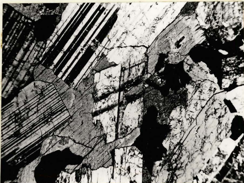
Figure 24. Gabbro, one mile northwest of Colter Lake. Note subophitic texture and the basal section of amphibole to the right of centre in the figure. Crossed nicols, X 26.
