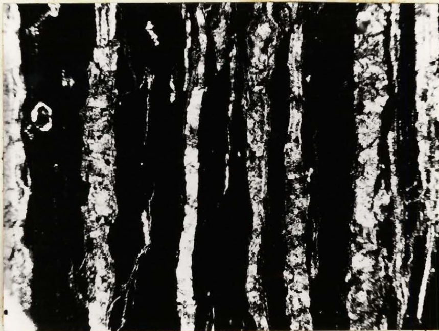
Figure 32. Iron formation. Thinly bedded manganiferous hematite from a metamorphosed section of the Iron Ore Hill deposit. The lighter bands in the figure are composed largely of manganocalcite and quartz, with minor amounts of chlorite and magnetite. Plain light, X 26.
