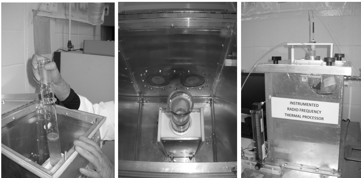
Figure 5-3 : Extraction of apple peel phenolic compounds using RFAE applicator
