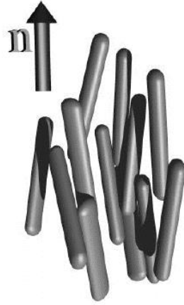
Figure 4 A schematic of rod-like building blocks of nematic phase and its characteristic director n .
