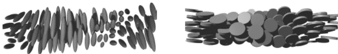
Figure 8 Schematics of helical director propagation in cholesteric phase for rod-shape molecules (left) and disc-like molecules (right). [6]
