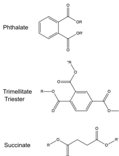
Figure 2. Chemical structure of plasticizers. Chemical structure for common plasticizers including phthalates (BBzP and DEHP), TOTM, and succinates (DOS and DHS)
