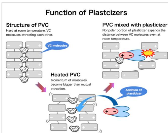
Figure 1. Function of Plasticizers. VC (vinyl chloride) is rigid at room temperature and maintains its shape. The introduction of plasticizers prevents VC molecules from coming close together, softening the material. Adapted from (1).
