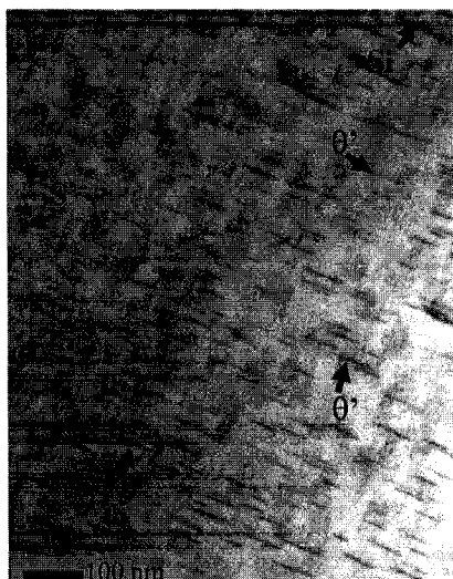
Figure 5.27 – High-Density Fine Precipitates Homogeneously on the \alpha Matrix Sample was Solution Heat Treated at 495 °C for 4 h and Aged for 4 h at 180 °C
