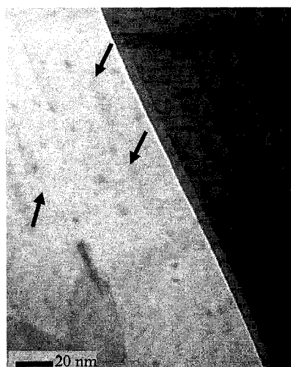
(e) Precipitation of \theta' and \theta After 12 h of Aging at 180 °C
