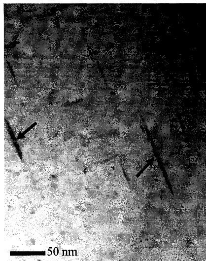
(c) Si Plates After 12 h of Aging at 180 °C
