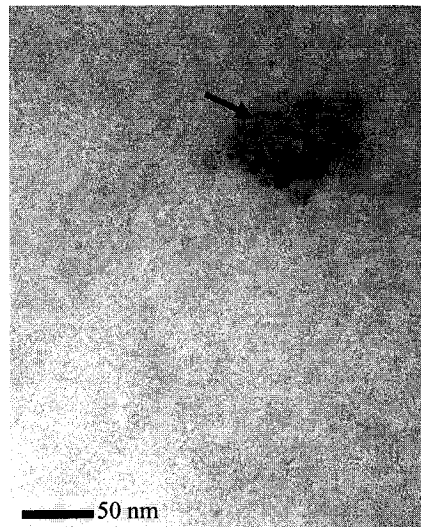
(a) Spherical Si Particle After Solution Treated at 495 °C for 4 h and Quenched in Water at 90 °C
