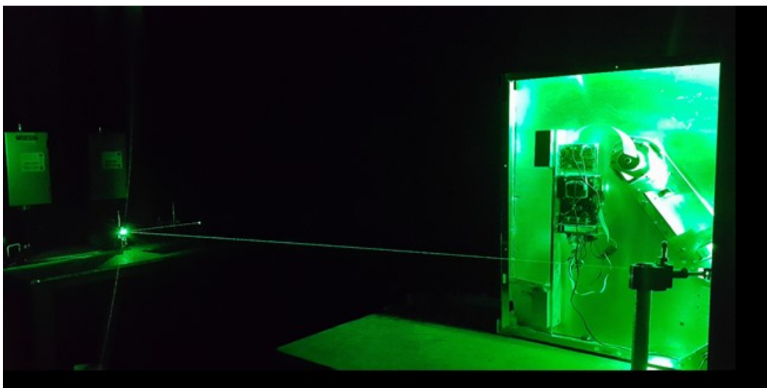
Figure 3.9 Operation of the directing mirrors and the laser scanning device
