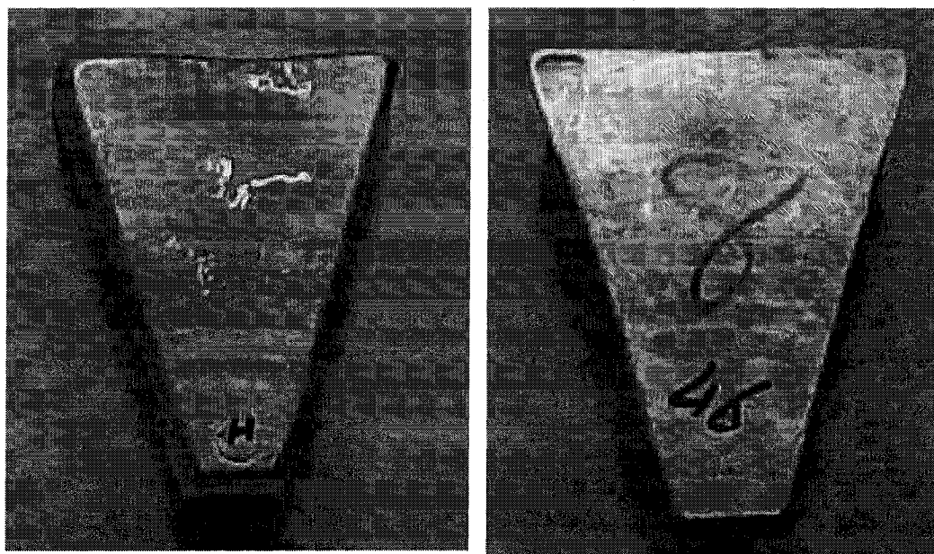
Figure 4.4. Magnesium casting produced without heat pipe cooling (H1)
