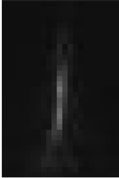
Figure 26 Point spread function of the customized OPM system obtained by using 200nm fluorescent beads (TetraSpeck) embedded in 1% agarose gel and imaged using 488nm laser with power at 20mW
