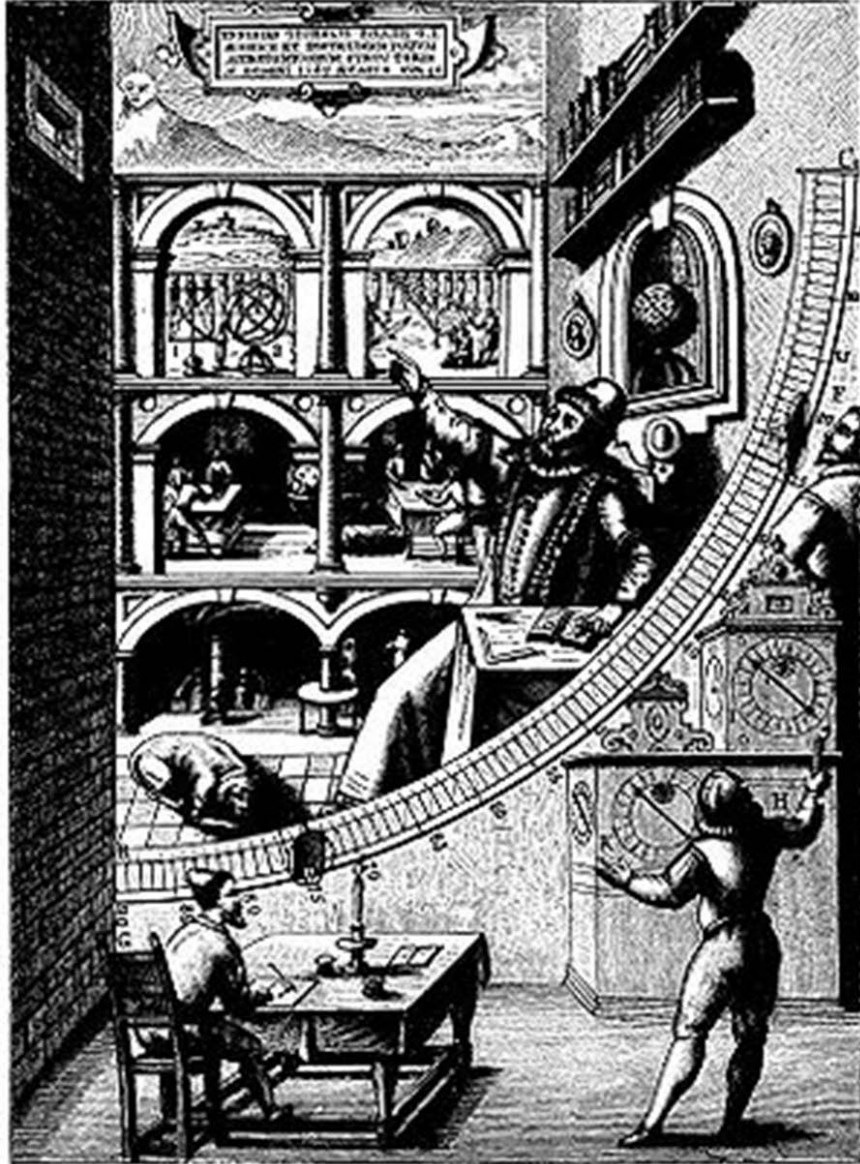
Figure 25. Tycho Brahe, Title page from Astronomiæ instauratæ mechanica (1598), illustrating Brahe's quadrant. Note the multiple portrayals of Brahe.
