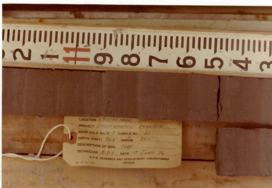
PLATE 2.8 CLOSEUP OF SECTION OF CORE SHOWN IN PLATE 2.7 (note, silt bands at 10.9 and 11.2)
