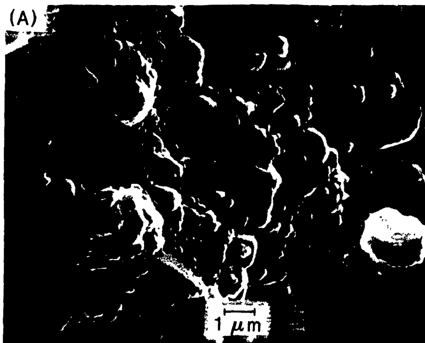
Figure 5.24: Top views of two layers of filter paper after being used to filter press (at 345 kPa) an A-17 slip. (A) First layer - 2.5 μm pore paper that was in contact with the cake.
