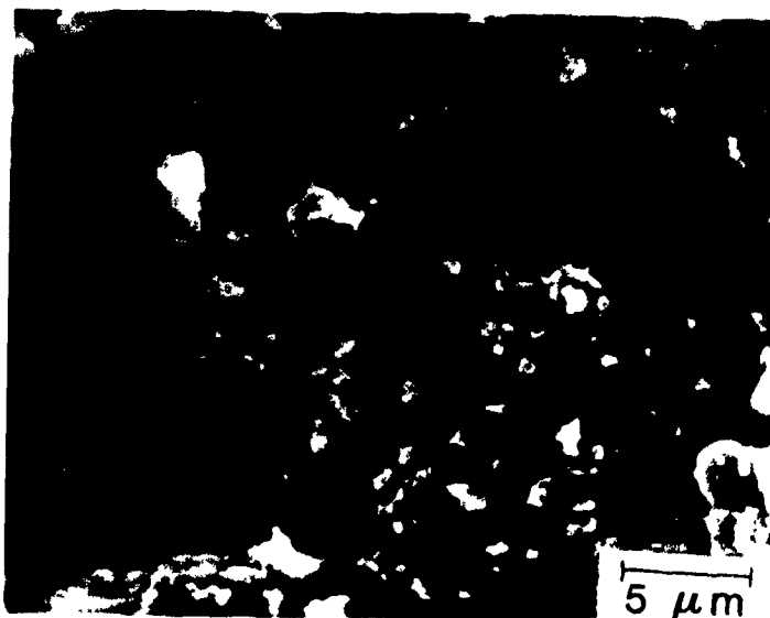
Figure 5.2: Top view of powder remaining on filter paper (90% C-71FG and 10% A-16SG, filter paper pore size = 2.5\ \mu\text{m} , and P = 345\ \text{kPa} )
