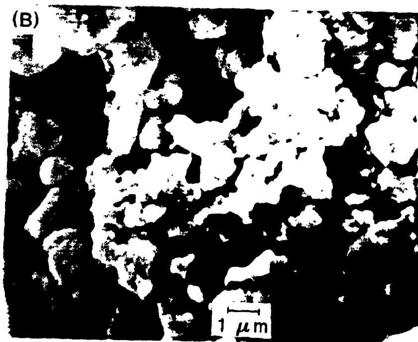
Figure 5.5: Longitudinal cross-sections (A) near the middle and (B) near the bottom surface of an A-17 cake. The cake was presintered at 1500 °C for one hour (filter paper pore size = 0.1 \mu\text{m} , and P = 345 \text{ kPa} ).
