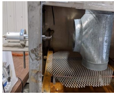
b. Inside view of steam chamber with horn and duct
