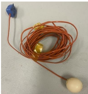
Figure 6.2. Nylon sphere with thermocouple
