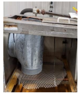
b. Inside view of steam chamber with horn and duct
