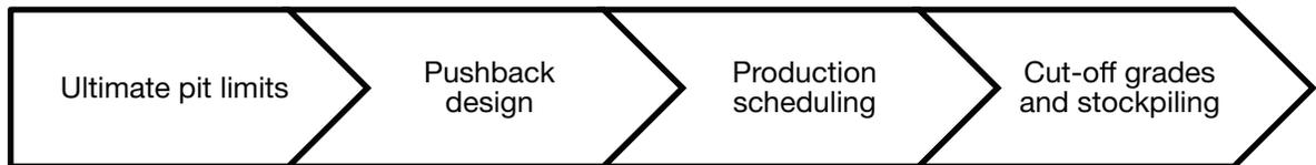
Figure 2–1: A traditional open pit framework for mine design and production scheduling.
