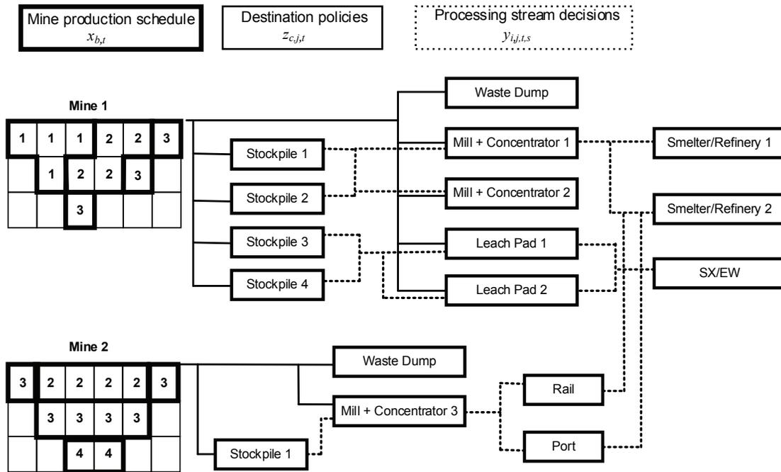
Figure 6–2: Decision variables related to material flowing through a mining complex.
