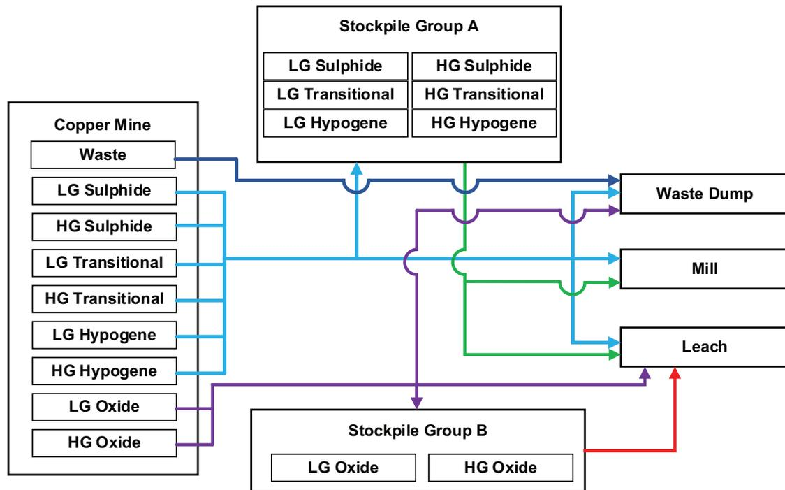
Figure 6-5: Material flow diagram for the copper mining complex.
