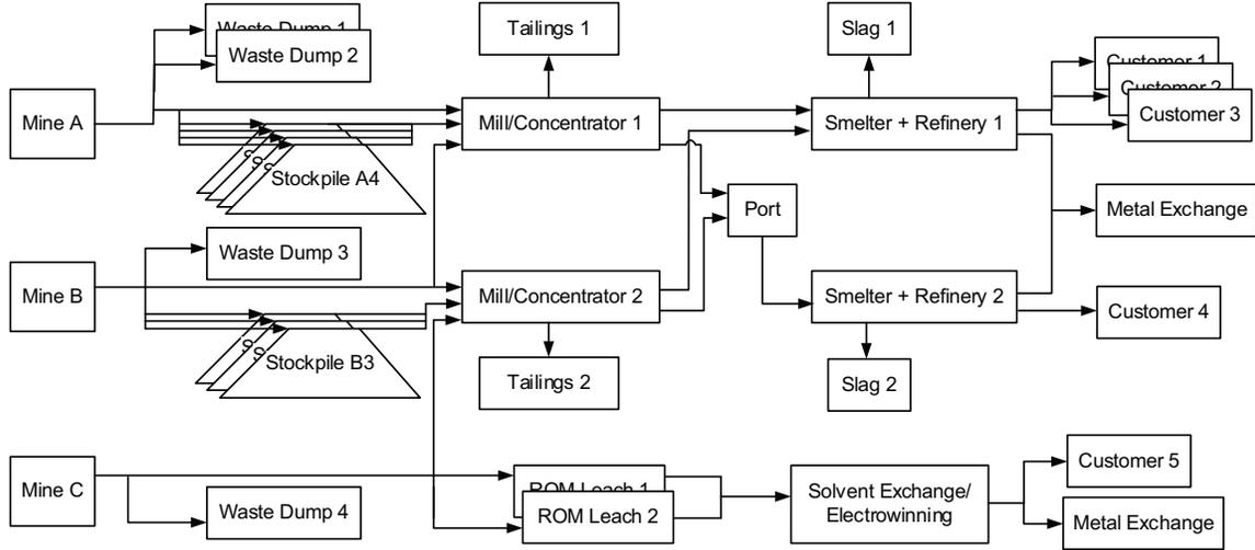
Figure 1–1: A hypothetical mining complex with multiple mines, processing streams and sales options.
