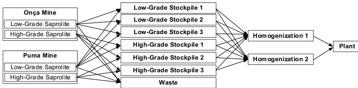
Figure 4–2: Flow of materials at the Onça Puma nickel laterite blending chain.
