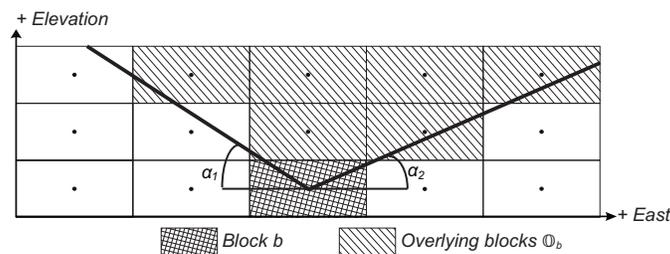
Figure 5-2: 2D example of blocks that must be uncovered ( $\mathbb{O}_b$ ) prior to extracting block  $b$ . Note that variable slope angles are defined for the West ( $\alpha_1$ ) and East ( $\alpha_2$ ) walls.
