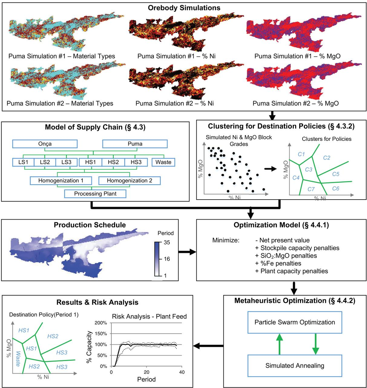
Figure 4-3: Overview of the proposed supply chain optimization methodology.
