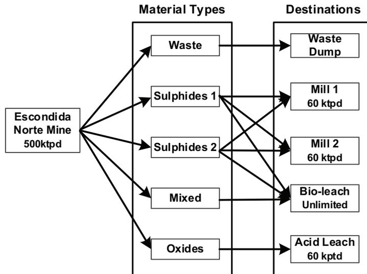
Figure 3–1: Flow chart of materials to various destinations at the Escondida Norte mining operation.
