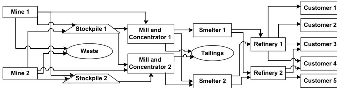
Figure 4–1: Hypothetical example of a mining supply chain.
