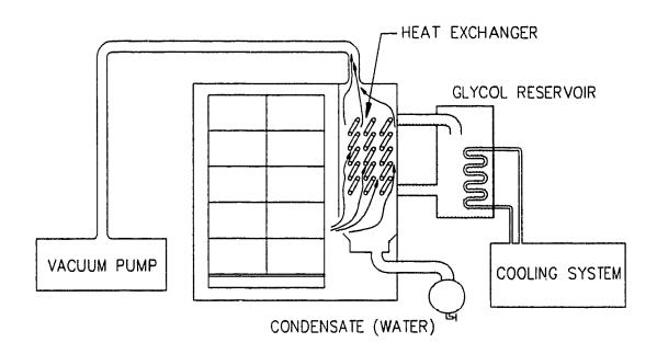
Figure 3.4: Schematic view of a vacuum cooler.
