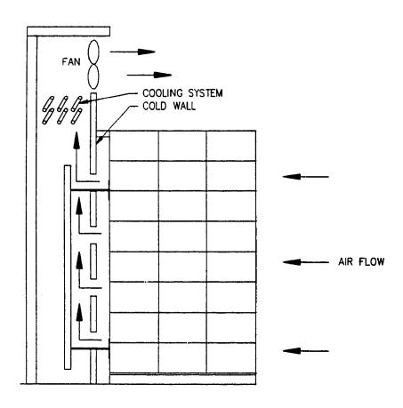
Figure 3.3: Schematic of the cross section of a cold-wall type forced-air cooler.
