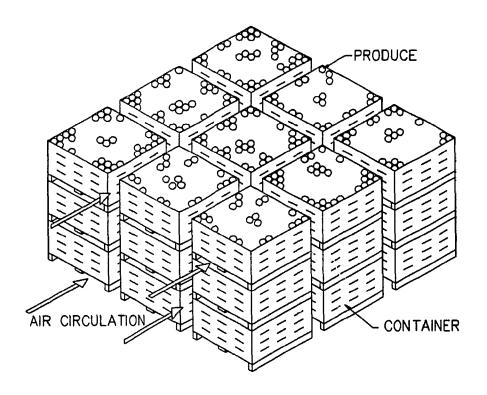
Figure 3.1: Schematic of the air circulation during room cooling.
