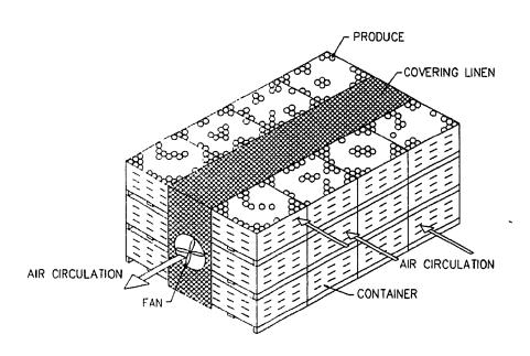
Figure 3.2: Schematic view of a forced-air cooling tunnel.
