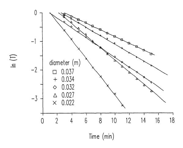
Figure 4.3: Ln(T) as a function of time for broccoli stalks of different diameters during the hydrocooling process.
