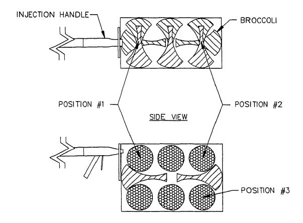
Figure 5.11: Typical box of 14 bunched broccolis where the three positions of the thermocouple are shown.
