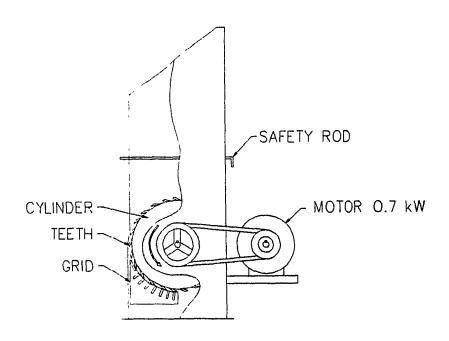
Figure 5.8: Ice crusher mounted with the type A grid.
