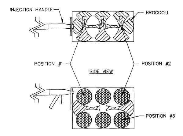
Figure 4.2: Typical box of 14 bunched broccolis bunched where the three positions of the thermocouples are shown.
