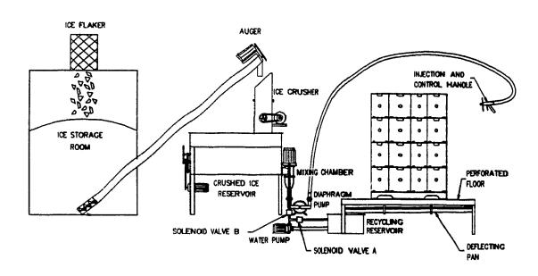
Figure 5.7: Schematic of the liquid-ice system developed during the project.
