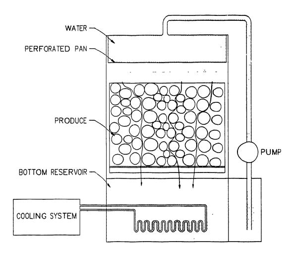
Figure 3.6: Schematic view of a hydrocooler.
