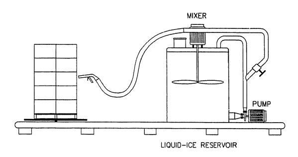
Figure 3.8: Conventional liquid-ice system producing 180 boxes per hour.
