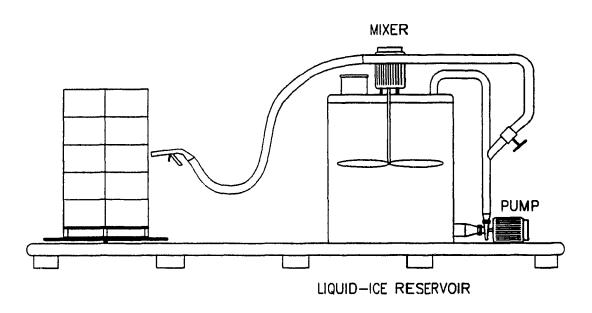
Figure 5.6: Conventional liquid-ice system producing 180 boxes per hour.
