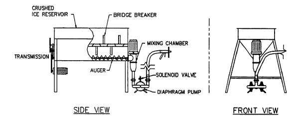
Figure 5.9: Schematic of the crushed ice reservoir and the mixing chamber.
