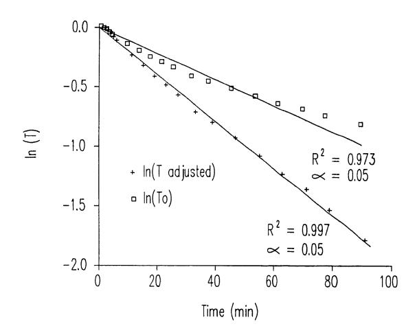
Figure 4.5:  $Ln(T_0)$  and  $ln(T_{Adjusted})$  as a function of time for a broccoli stalk during the cooling process.
