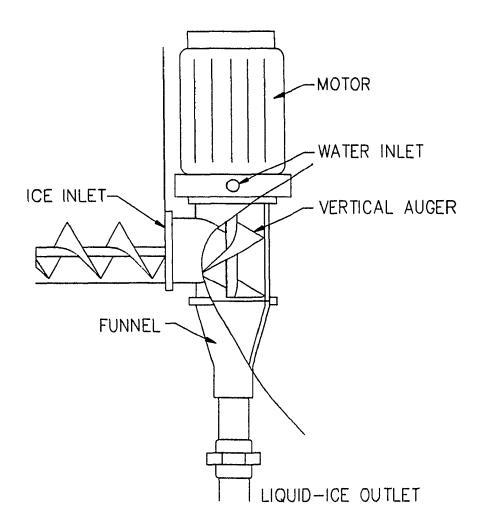
Figure 5.10: Schematic of the mixing chamber used with the liquid-ice system.
