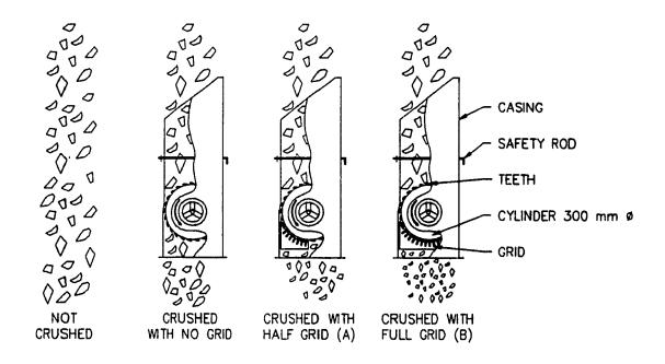
Figure 4.1: Schematic of the crusher assembly used to obtain the four different ice particle sizes.
