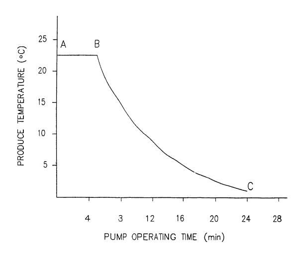
Figure 3.5: Typical temperature variation during vacuum cooling process.
