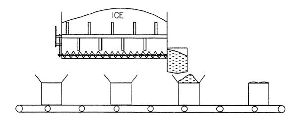
Figure 3.7: Automatic icing package system.
