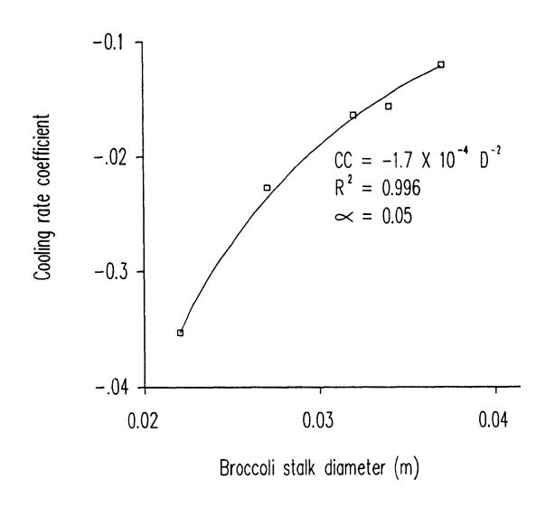
Figure 4.4: Cooling coefficient as a function of the diameter for broccoli stalks during the hydrocooling process.
