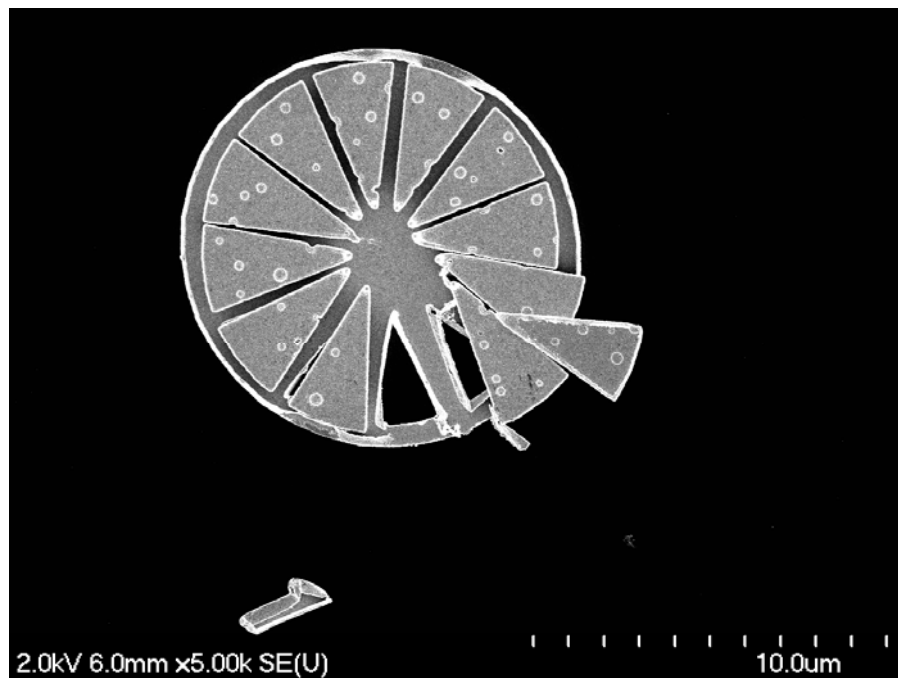
Figure 25 Example of incomplete lift-off from sample 1
