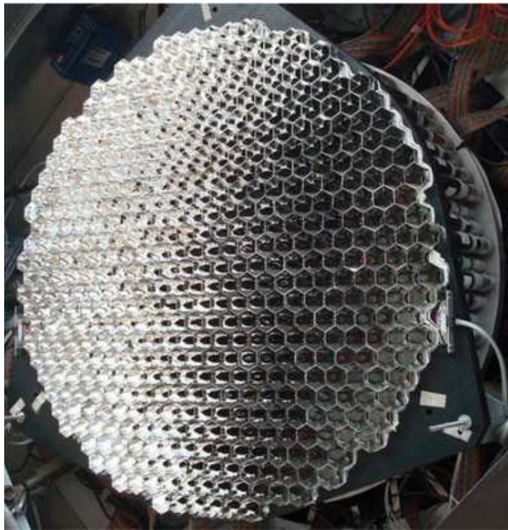
Figure 2–5: Telescope camera with the shutter open. The lightcones are deployed in front of the pixels. Image source: Sean Griffin.
