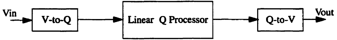
Figure 4.8: The SC Technique from a Charge Processing Point of View
