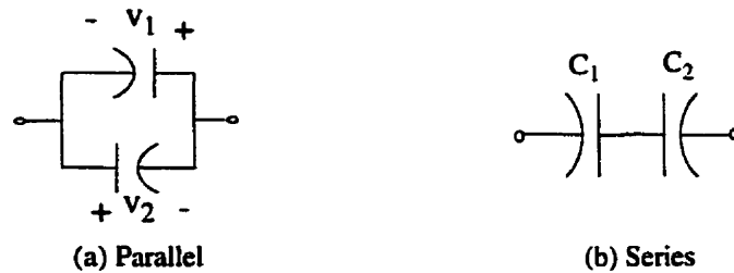
Figure 4.14: Structures to Reduce Non-Linearity, without DC Biasing
