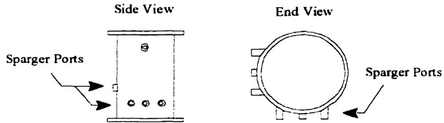
Figure 3-2: Schematic of sparger configuration at the bottom of the pilot column.
