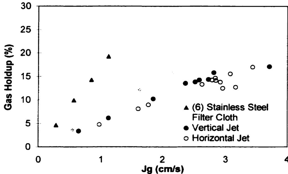
Figure 4-3: Gas holdup trends of pilot column bubble generating devices
