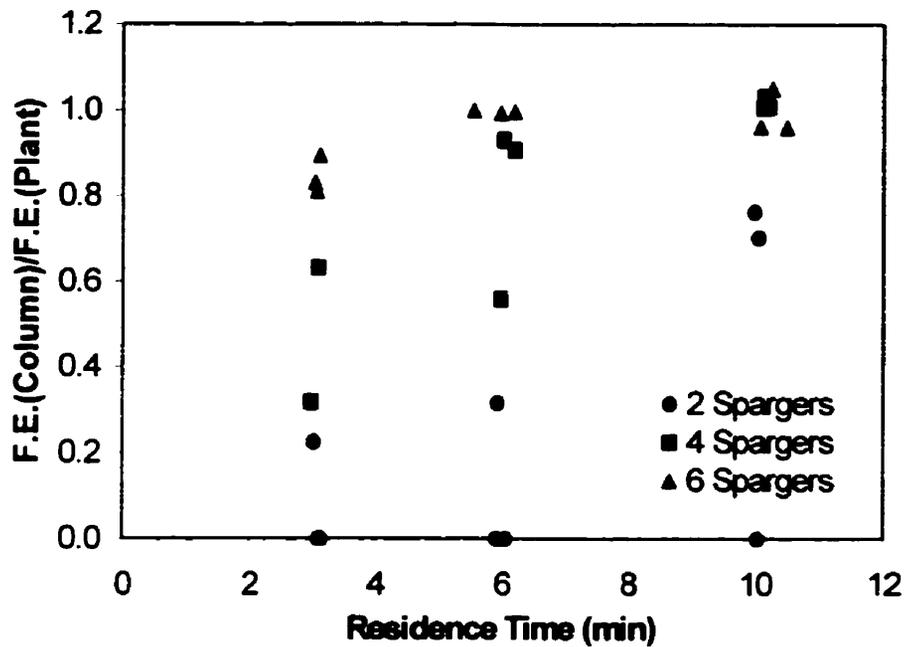
Figure 4-1: Flotation performance versus residence time for the pilot column using ss spargers (various  $J_g$ ).
