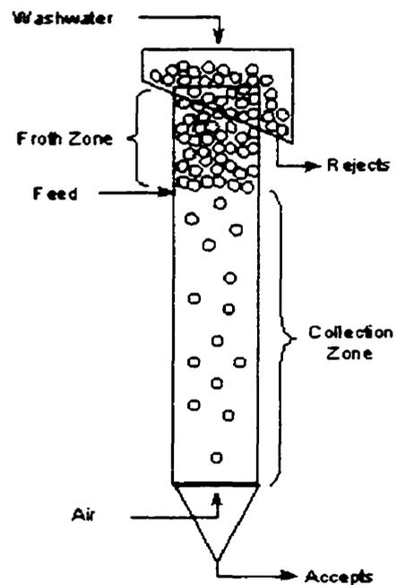
Figure 1-1: Schematic of a flotation column. (Terminology refers to use in the paper deinking industry).
