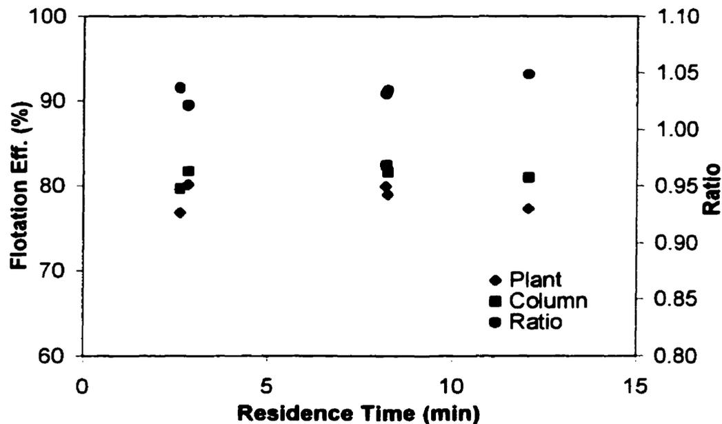
Figure 4-1: Flotation efficiency of lab column using accepts from Voith cells as feed.
