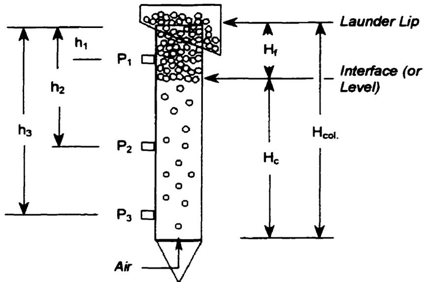
Figure 3-1: Diagram of relative heights of the pressure transducers ( $P_1$  to  $P_3$ ) and the interface between the froth and collection zone.
