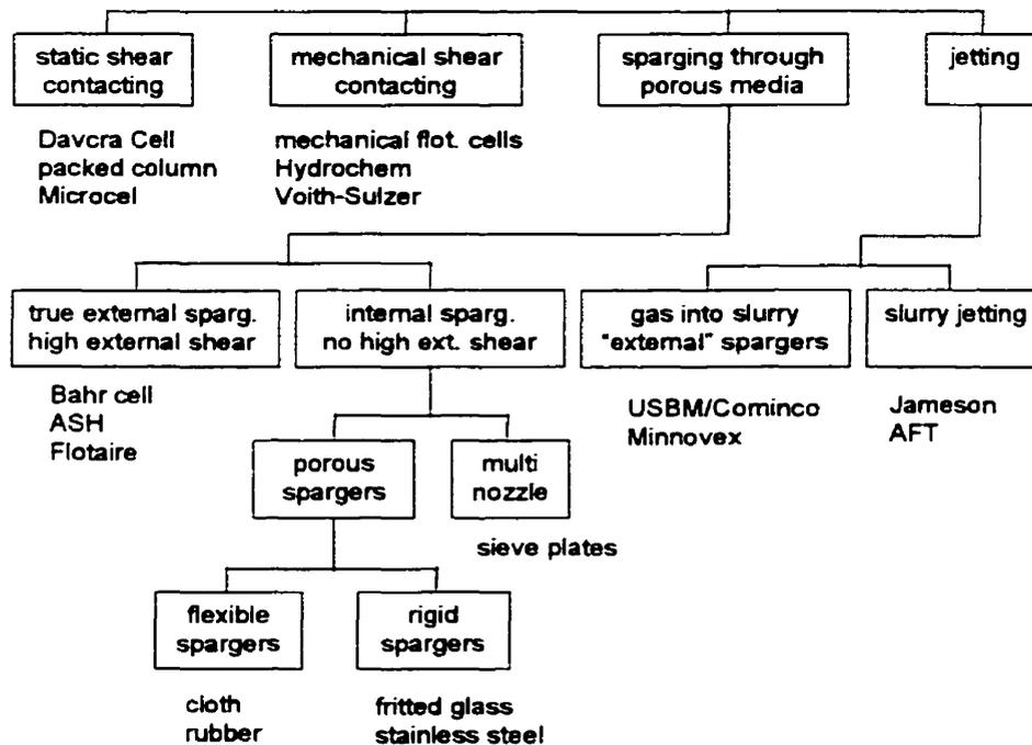
Figure 1-1: Bubble generating techniques (adapted from Paleari, 1993)
