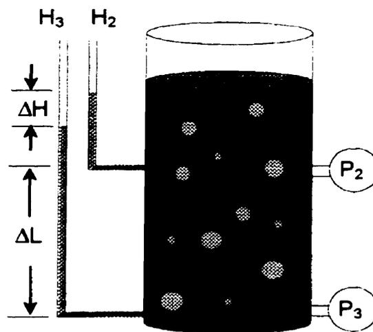
**Figure 3-1: Schematic of gas holdup measurement**
