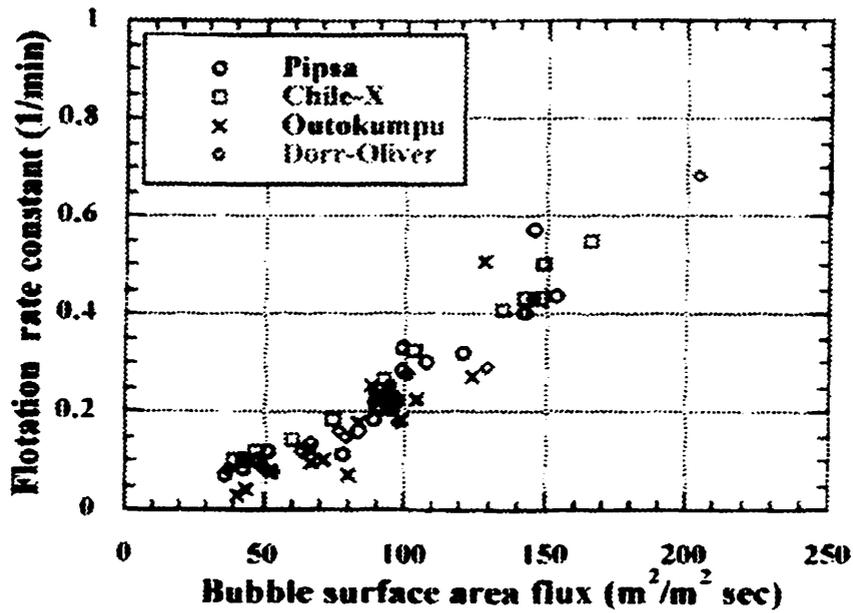
Figure 2-3: Overall flotation rate constant versus S<sub>b</sub> for four different impeller configurations on a mechanical float cell operating as a zinc cleaner [Gorain *et al.*, 1997].
