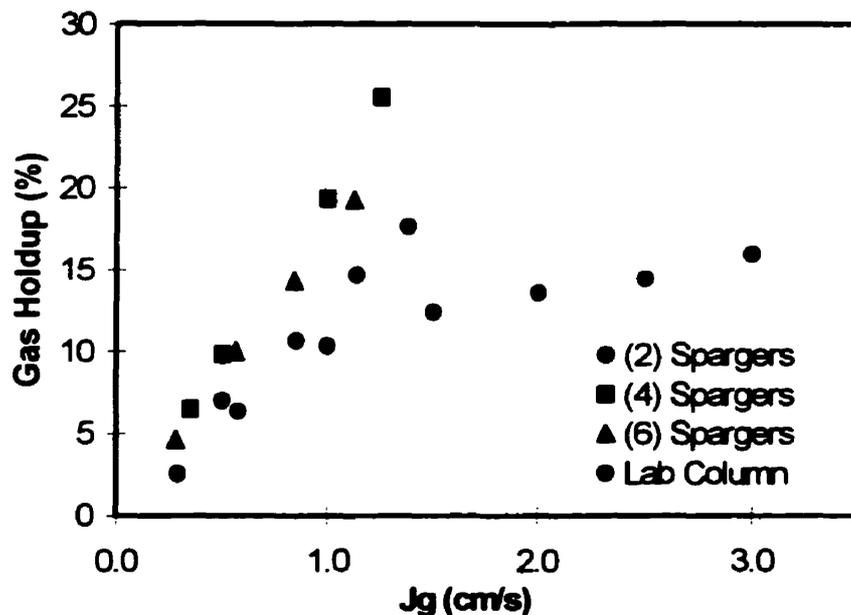
Figure 4-1: Gas holdup versus  $J_g$  for ss spargers in batch conditions using water and 30 ppm Dowfroth
