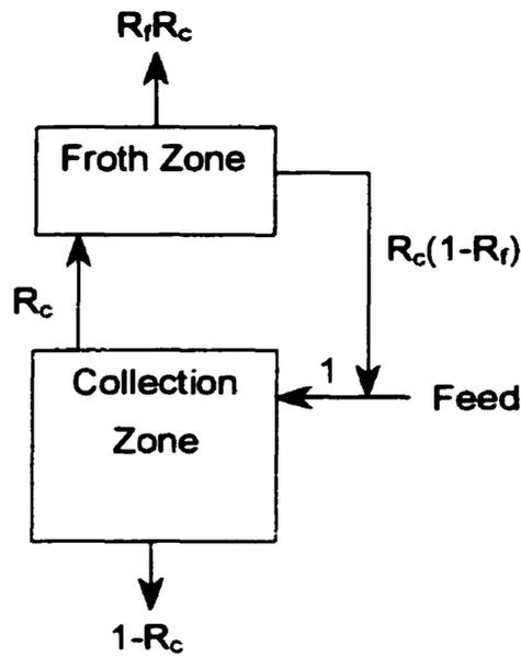
Figure 2-1: Schematic of froth and collection zone recovery in a flotation column [Finch and Dobby, 1990].
