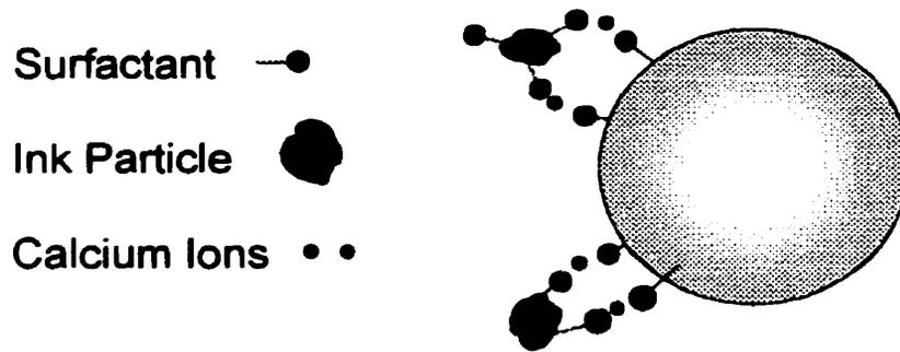
Figure 2-1: Schematic model of air bubble -- particle attachment in a deinking system.
