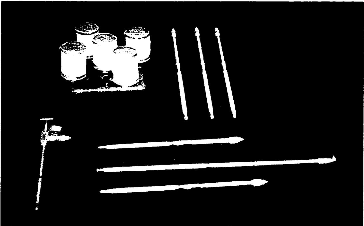
Figure 3-3: Jetting, filter cloth and stainless steel spargers (l to r)
