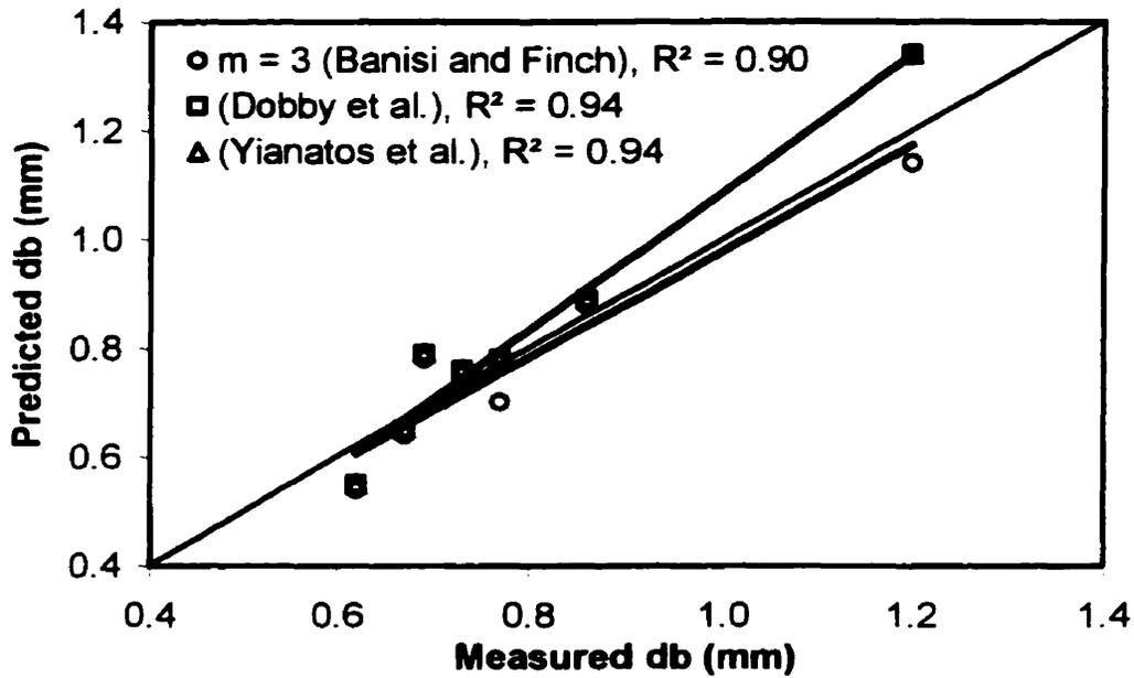
Figure 2-1: Comparison of measured db (photographic) to predicted db for three drift flux calculation methods (data from Banisi and Finch, 1994).
