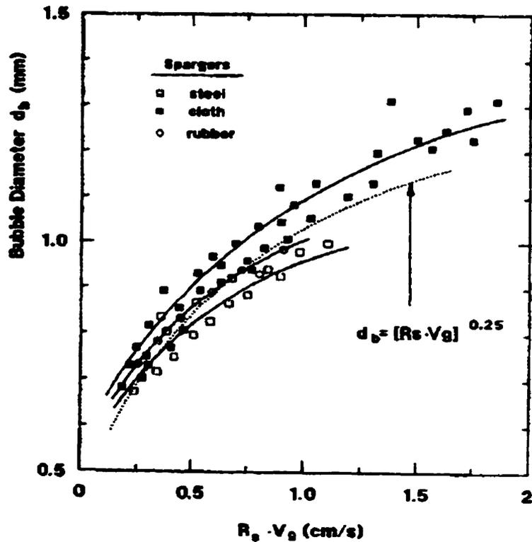
Figure 2-5: Effect on  $d_b$  of  $R_s$  and superficial gas velocity for steel, cloth, and rubber spargers [Xu and Finch, 1989]
