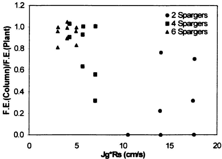
Figure 4-2: Flotation performance of the pilot column using ss spargers.
