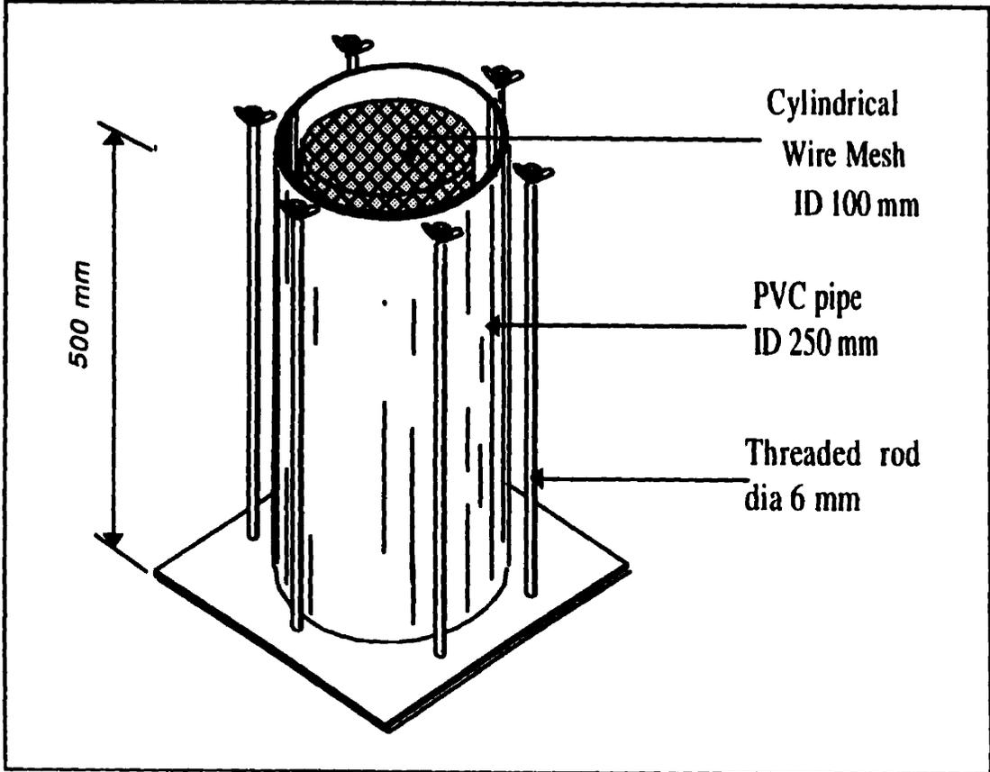
Figure 4.3 Storage Chamber with a Cylindrical Wire Mesh
