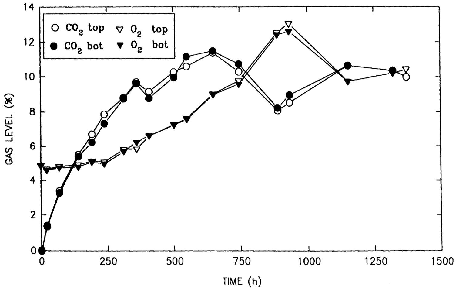
Figure 5.22 Comparison of Gas Sampled from Top and Bottom of the Storage Chambers with Diffusion Channel of 0.043 m and CSA of  $9 \times 10^{-6} \text{ m}^2$  as a Function of Time.
