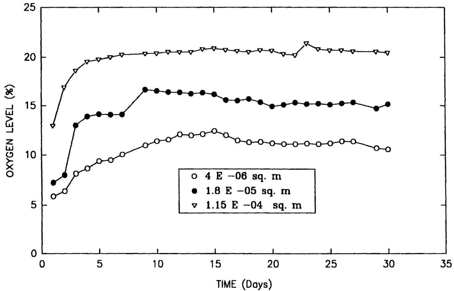
figure 5.16 Comparison of Progression of  $O_2$  for Chambers with Channels of 0.03 m Length and Three Varying Cross Sectional Areas.
