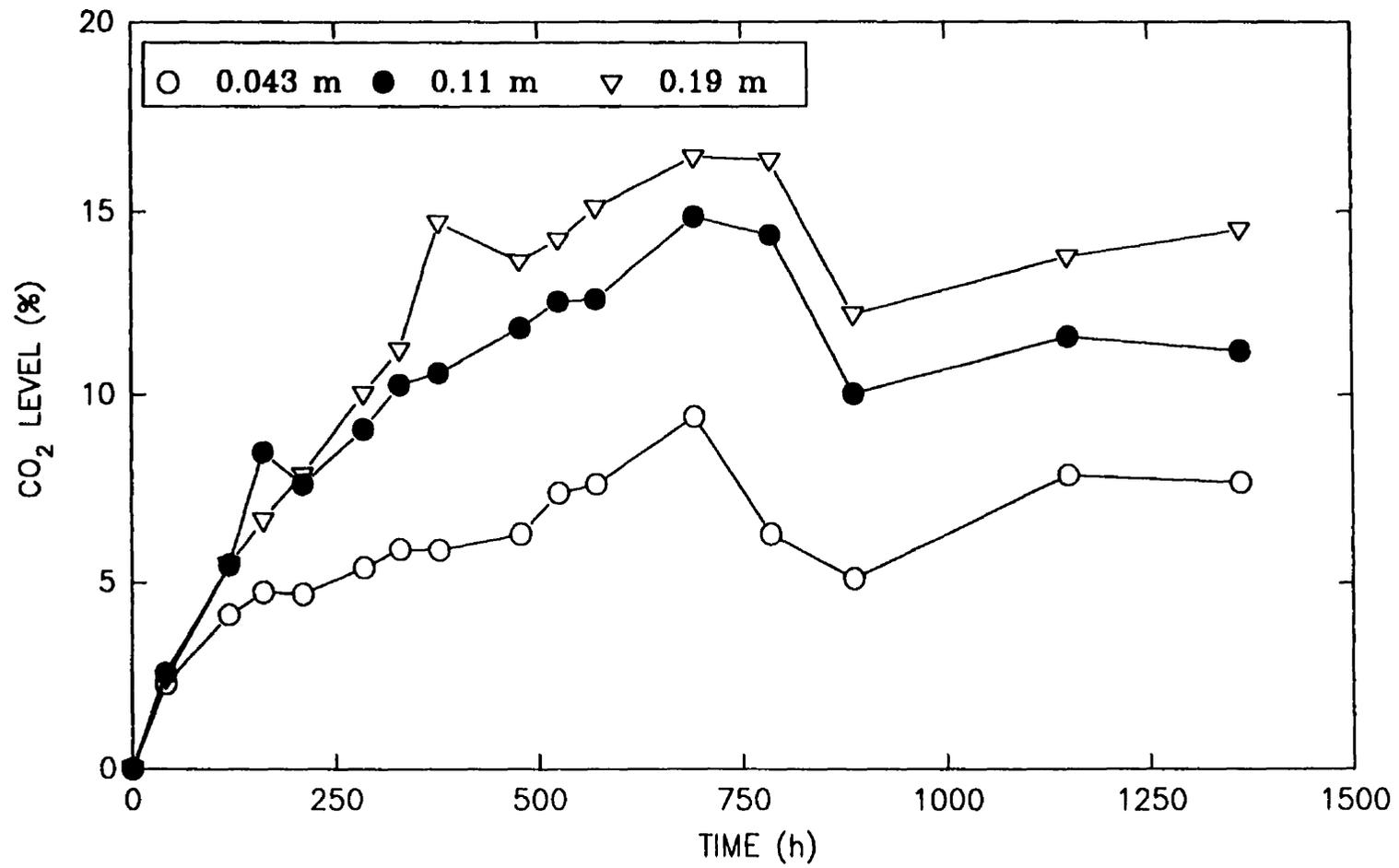
Figure 5.29 Progression of CO<sub>2</sub> in Chambers with Channels of Three Varying Lengths and CSA of  $4 \times 10^{-5} \text{ m}^2$ .
