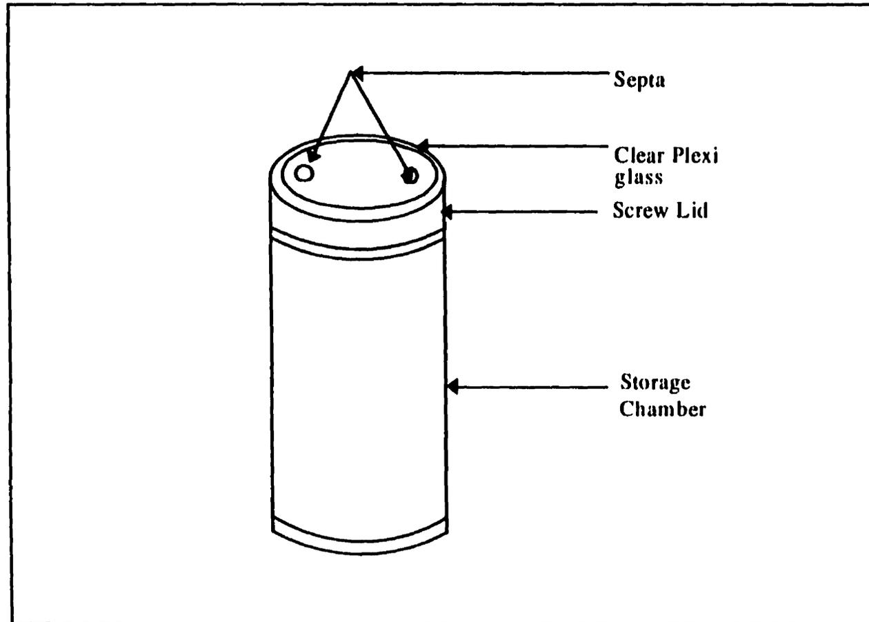
Figure 4.1 Schematic Diagram of the Storage Chamber for Measuring Respiration Rate of Spinach
