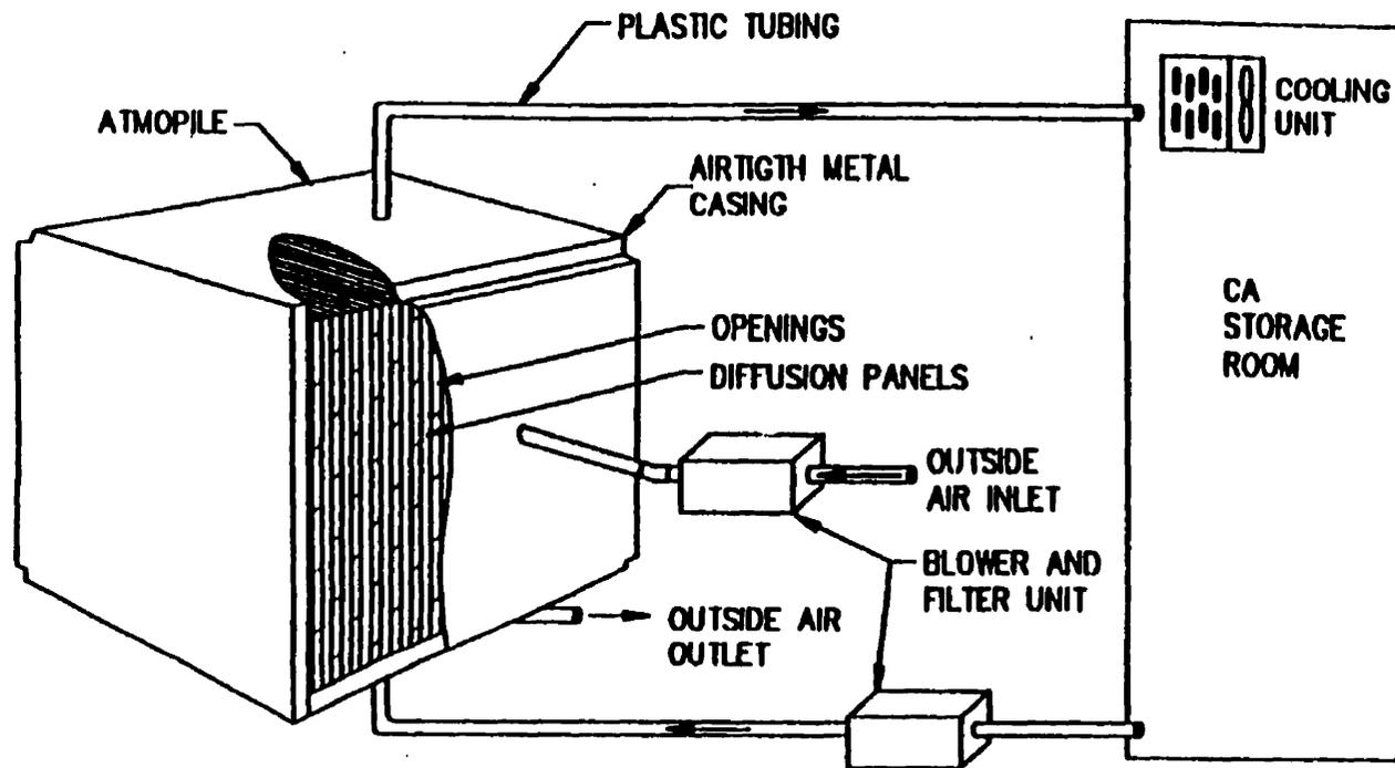
Figure 2.5 Schematic Diagram of The Atmolysair Membrane System (Raghavan and Gariépy, 1982)
