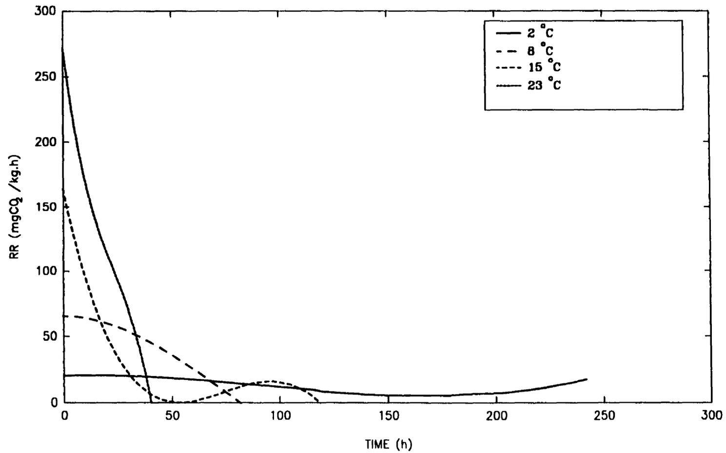
**Figure 5.1** Respiration Rate of Spinach at Four Levels of Storage Temperature with Time.
