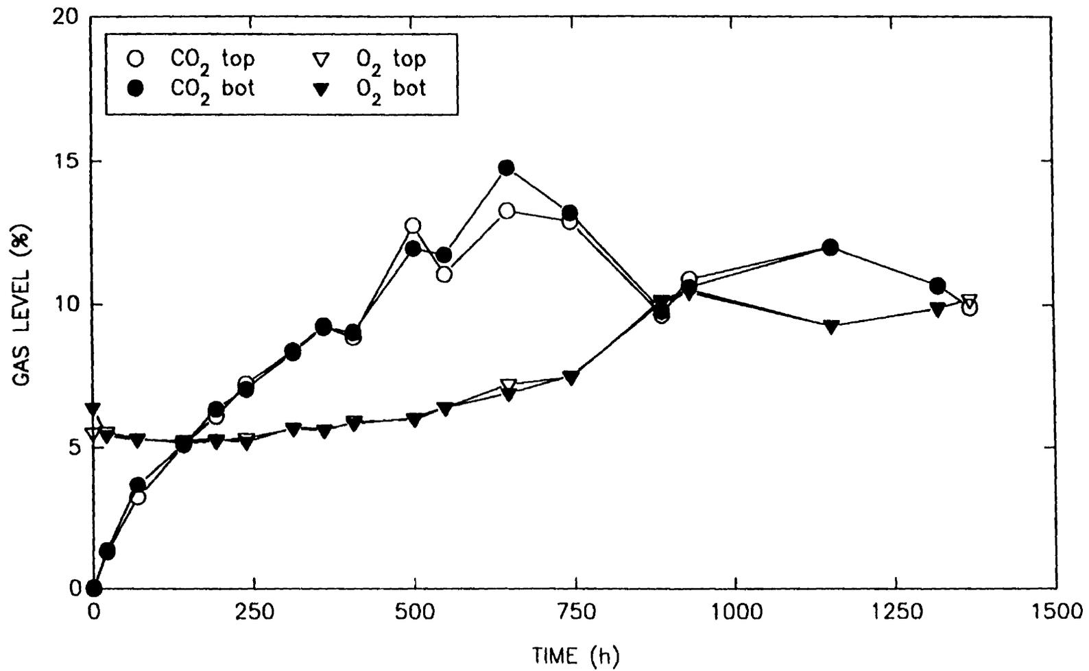
Figure 5.23 Comparison of Gas Sampled from Top and Bottom of the Storage Chambers with Diffusion Channel of 0.11 m and CSA of  $9 \times 10^{-6} \text{ m}^2$  as a Function of Time.
