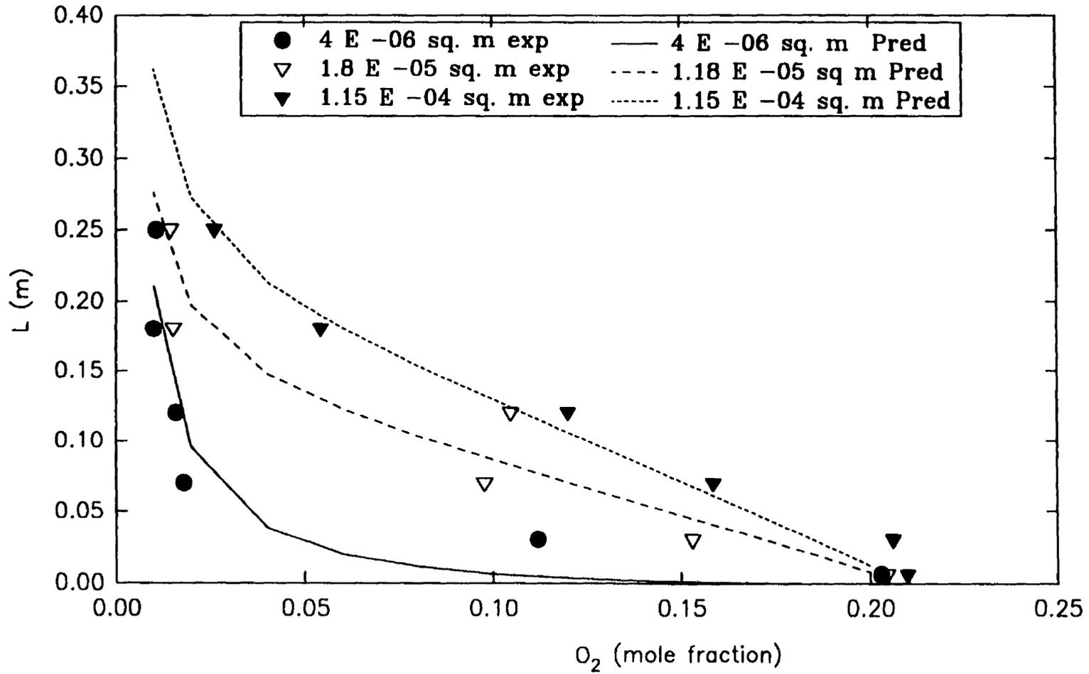
Figure 5.31 Comparison of Predicted Length of Diffusion Channel with Experimental Data for Three Varying Cross Sectional Areas.
