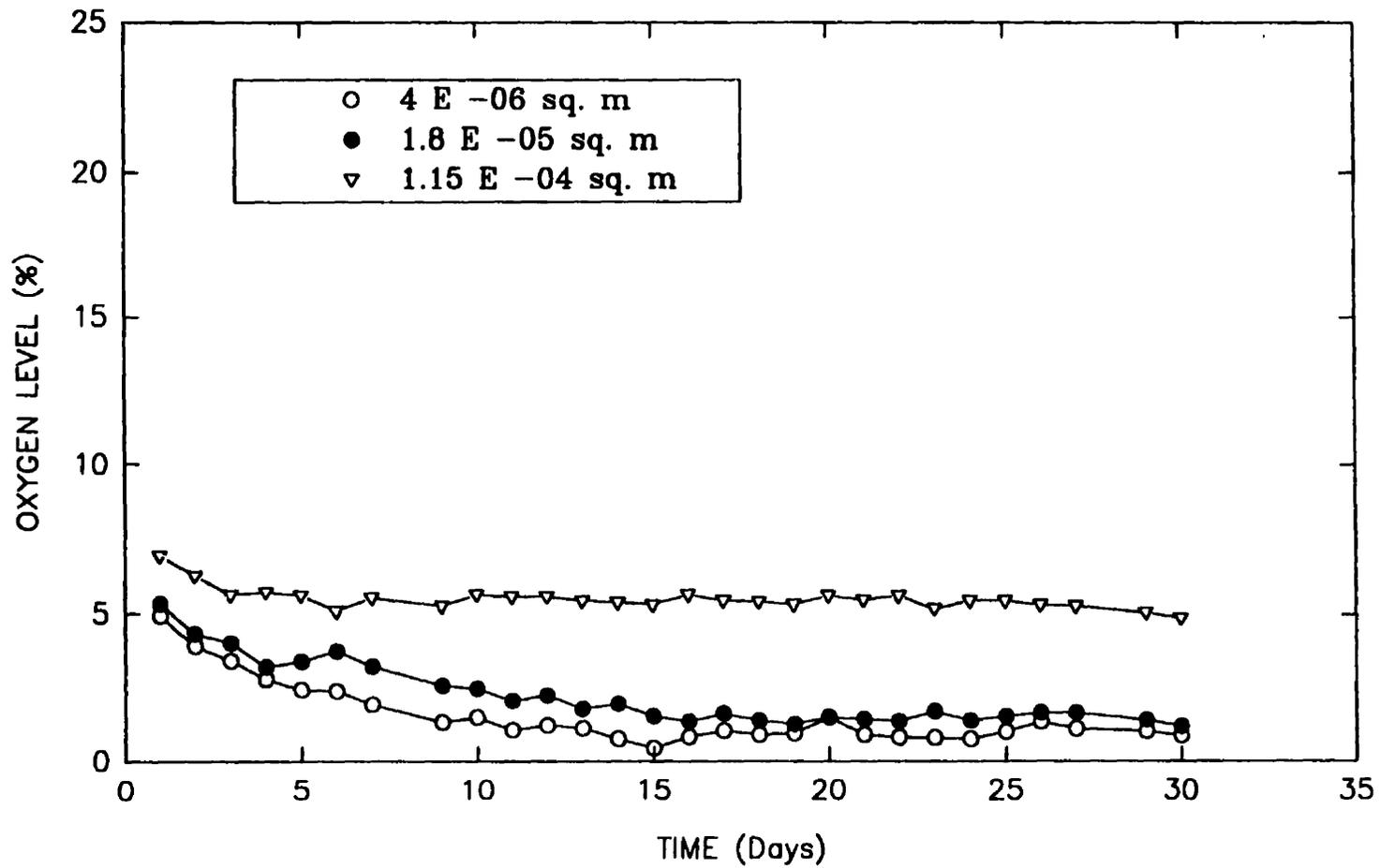
Figure 5.19 Comparison of Progression of  $O_2$  for Chambers with Channels of 0.18 m in Length and Three Varying Cross Sectional Areas.
