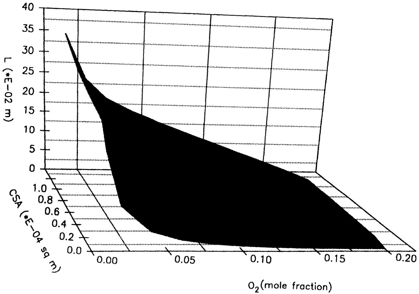
Figure 5.21 The Relationship of Length, Cross Sectional Area of Diffusion Channel and O<sub>2</sub> Steady State Level.
