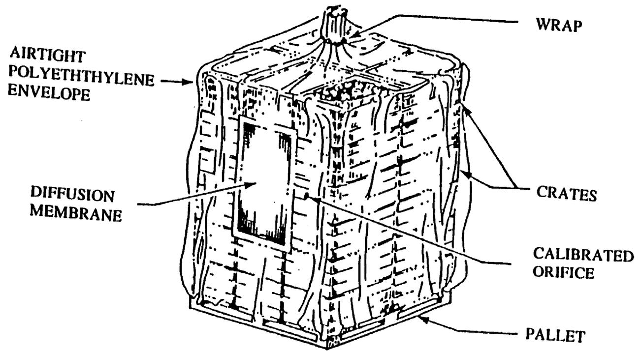
Figure 2.3 Diagram of The Pallet Package Membrane System.
