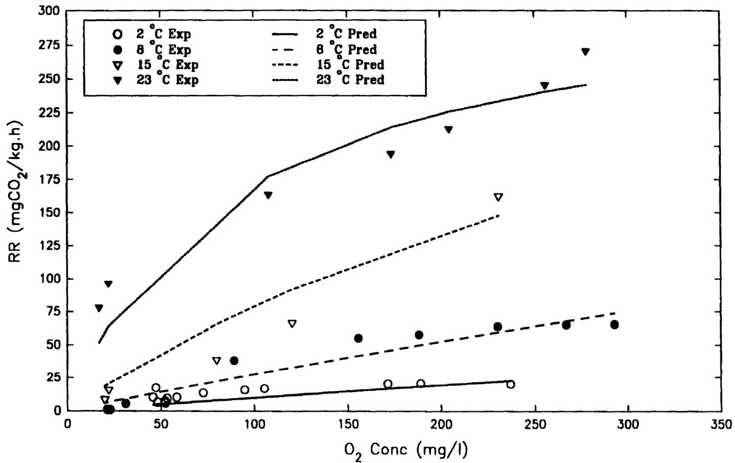
Figure 5.11 Comparison of Predicted and Experimental Respiration Rate of Spinach Calculated on O<sub>2</sub> consumption Rate as a Function of O<sub>2</sub> Concentration.
