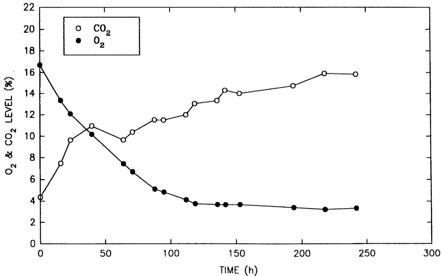
Figure 5.2 Progression of O<sub>2</sub> and CO<sub>2</sub> in Sealed Storage Chambers at 2°C as a Function of Time.
