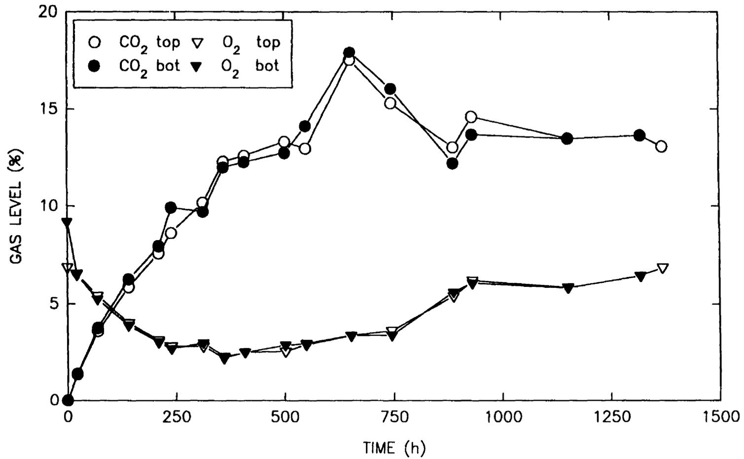
**Figure 5.24** Comparison of Gas Sampled from Top and Bottom of the Storage Chambers with Diffusion Channel of 0.19 m and a CSA of  $9 \cdot 10^{-6} \text{ m}^2$  as a Function of Time.
