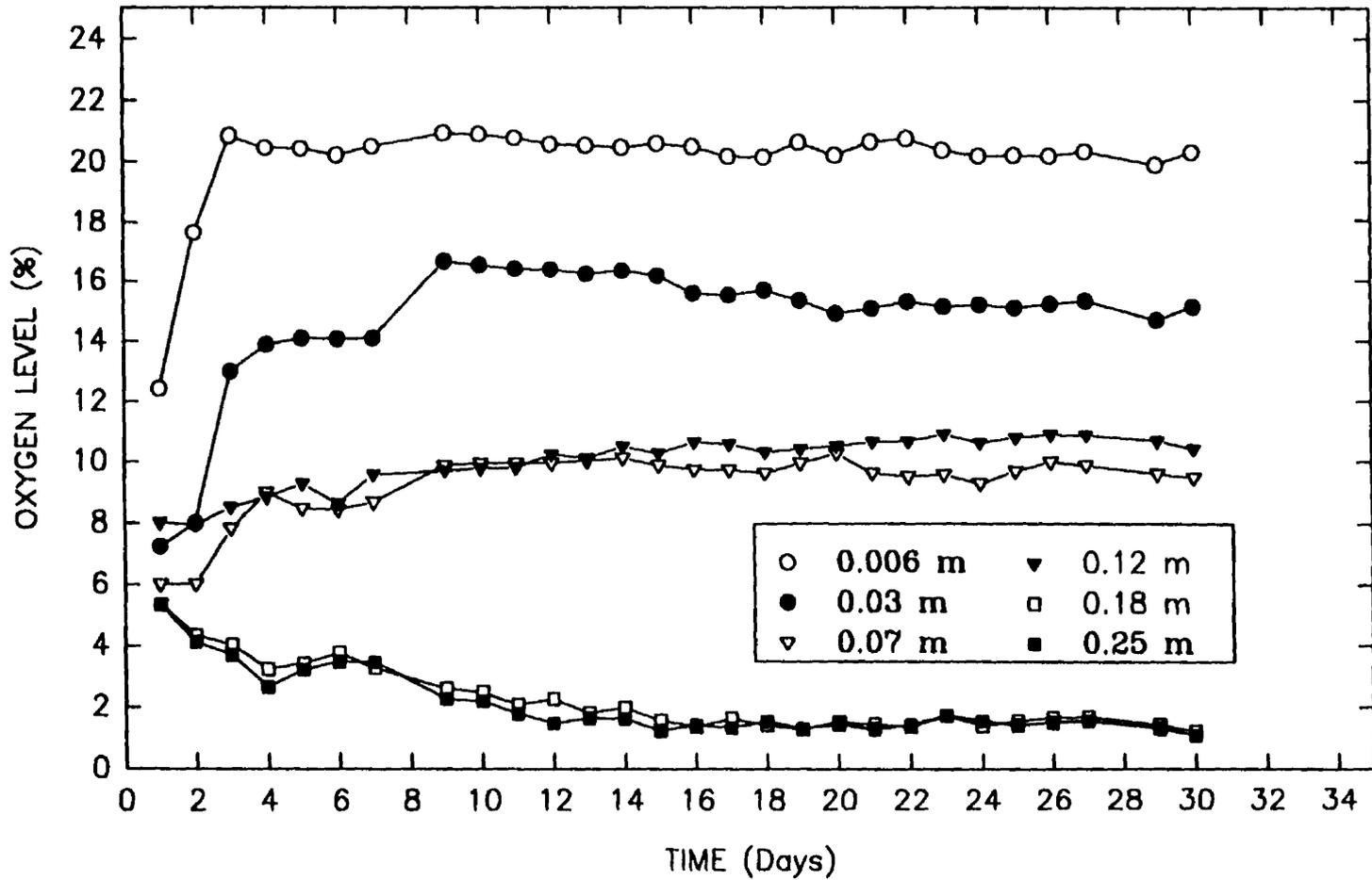
Figure 5.13 Progression of  $O_2$  in Chambers with Channels of Six Varying Lengths and a CSA of  $1.8 \cdot 10^{-5} \text{ m}^2$
