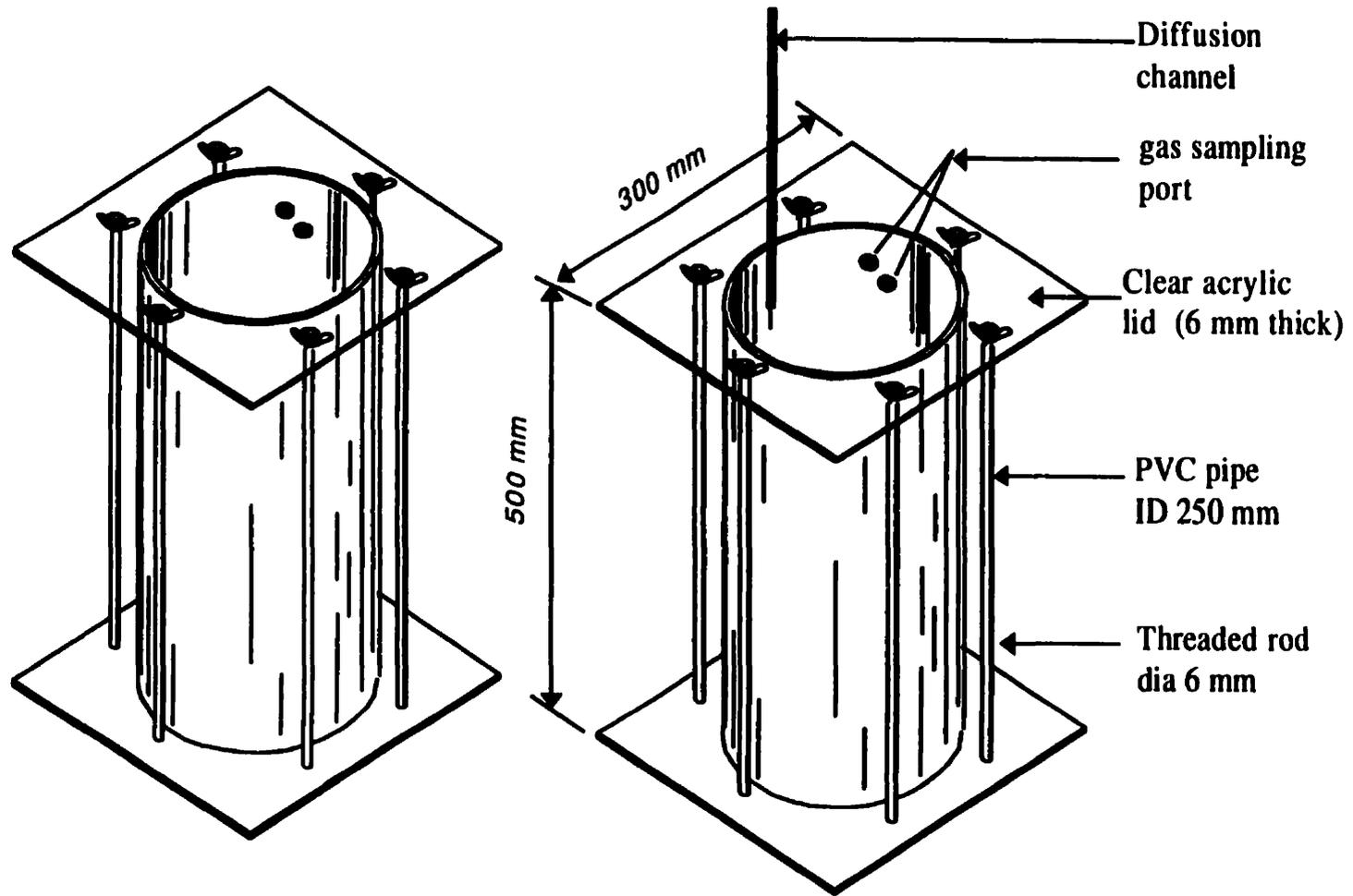
Figure 4.2 Schematic Diagrams of the Experimental Storage Chambers (with and without diffusion channel)
