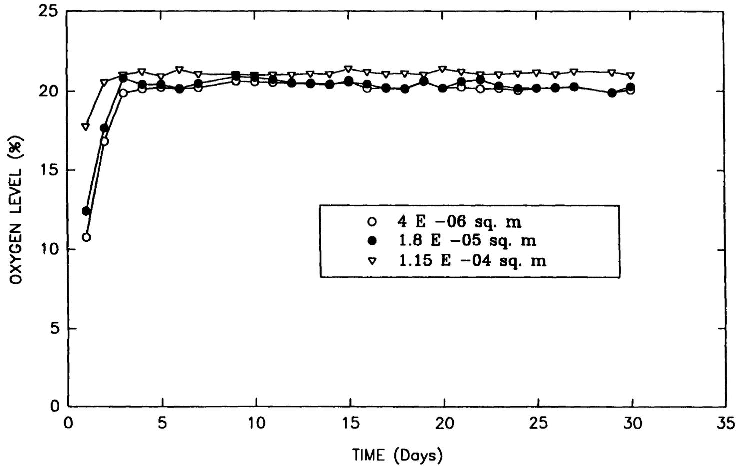
Figure 5.15 Comparison of Progression of  $O_2$  for Chambers with Channels of 0.006 m in Length and Three Varying Cross Sectional Areas.
