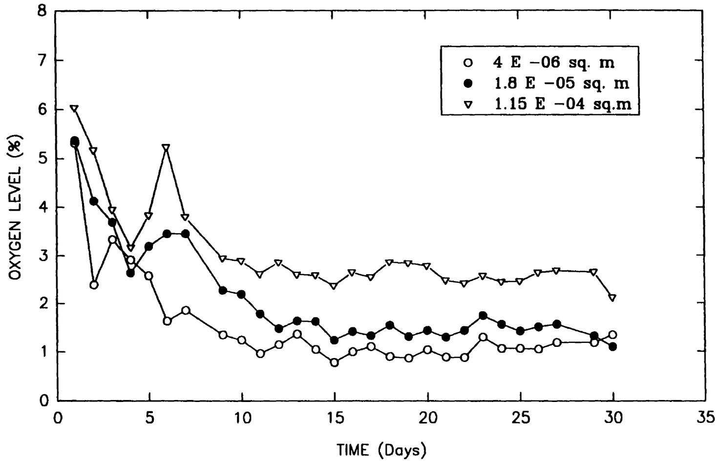
**Figure 5.20 Comparison of Progression of  $O_2$  for Chambers with Channels of 0.25 m in Length and three Varying Cross Sectional Areas.**
