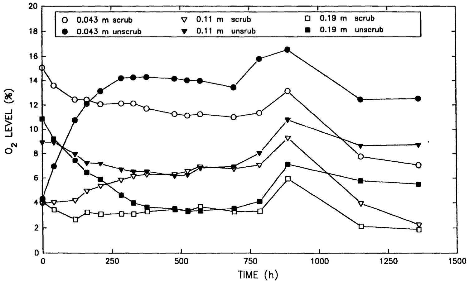
Figure 5.26 Comparison of O<sub>2</sub> Levels in CO<sub>2</sub> Scrubbed and Unscrubbed Chambers for CSA of  $4 \cdot 10^5 \text{ m}^2$ .
