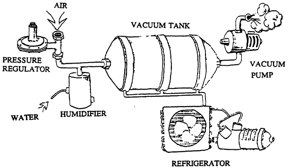
Figure 2.1a Schematic Diagram of a Hypobaric System
