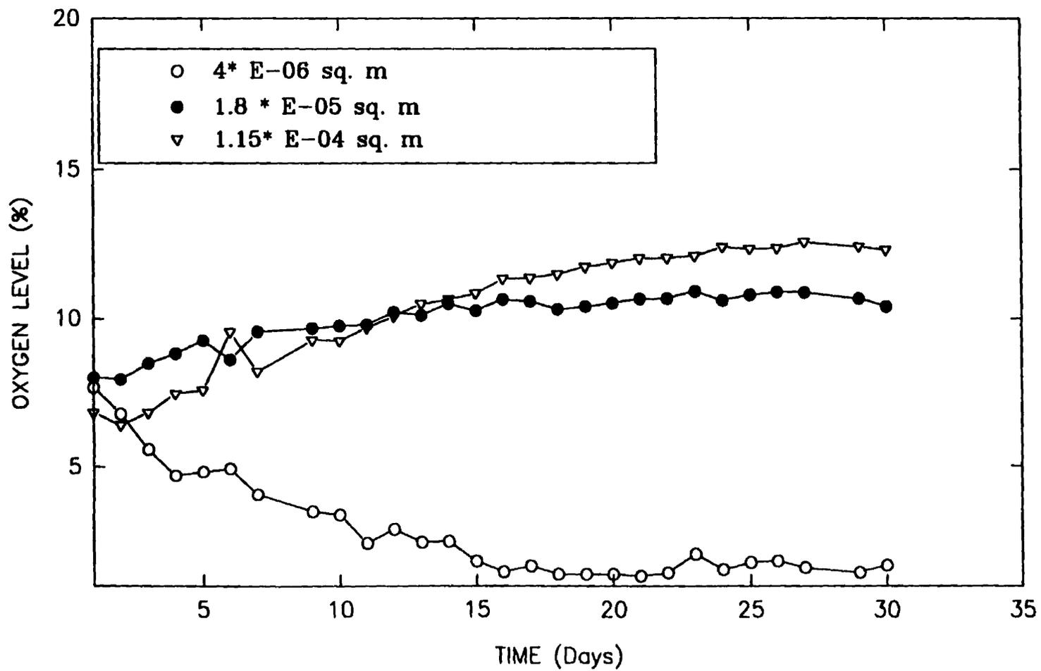
Figure 5.18 Comparison of Progression of  $O_2$  for Chambers with Channels of 0.12 m in Length and Three Varying Cross Sectional Areas.
