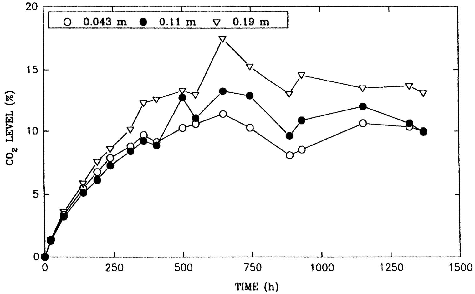
Figure 5.28 Progression of CO<sub>2</sub> in Chambers with Channels of Three Varying Lengths and CSA of  $9 \times 10^{-6} \text{ cm}^2$ .
