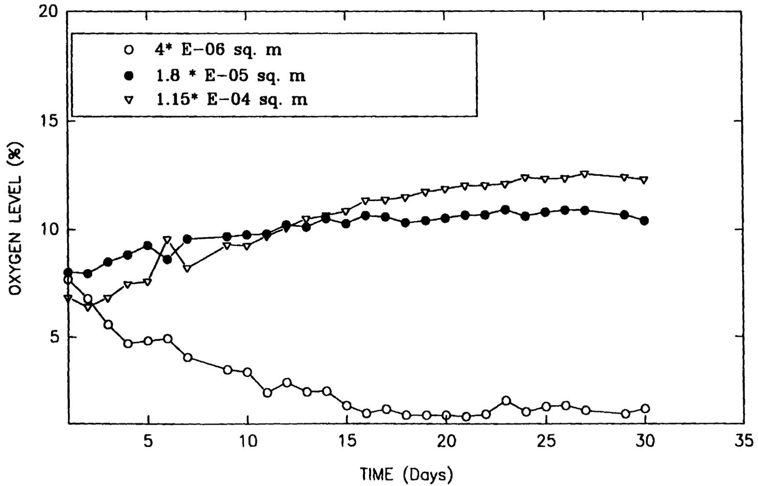
**Figure 5.18 Comparison of Progression of O<sub>2</sub> for Chambers with Channels of 0.12 m in Length and Three Varying Cross Sectional Areas.**
