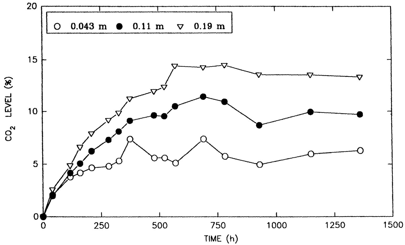
Figure 5.30 Progression of CO<sub>2</sub> in Chambers with Channels of Three Varying Lengths and CSA of 1.7\*10<sup>-4</sup> m<sup>2</sup>.
