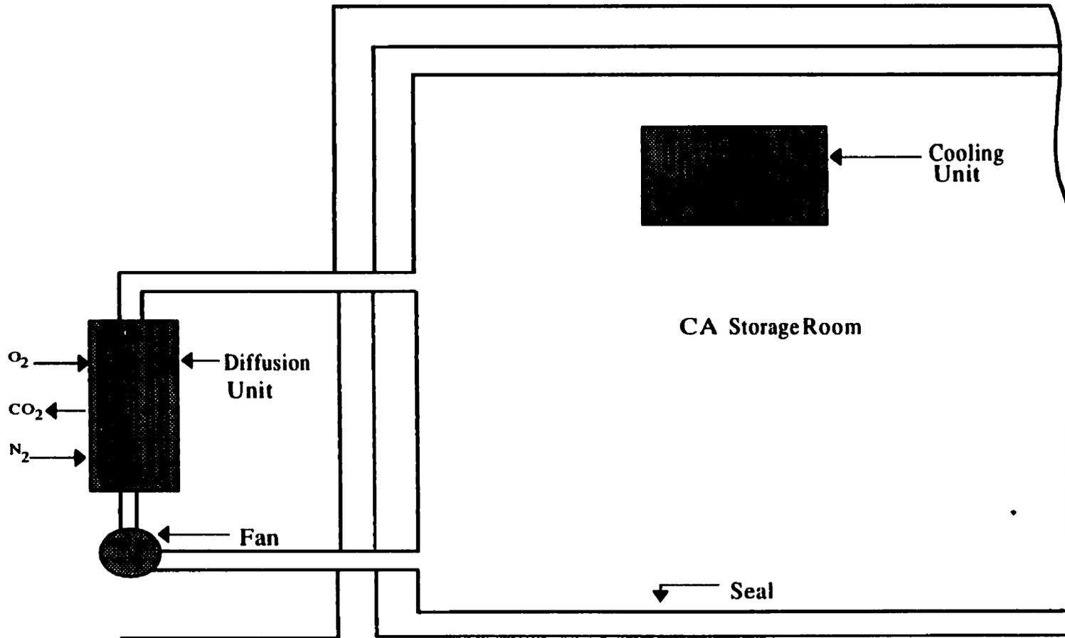
Figure 2.4 Schematic Diagram of the Marcellin Membrane System Installed Outside CA Room (Raghavan and Gariépy, 1985)
