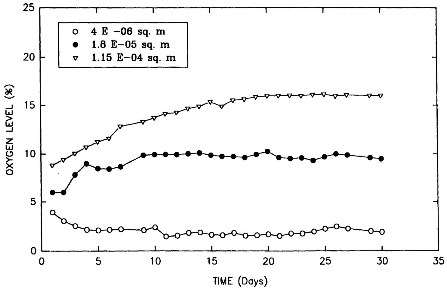
Figure 5.17 Comparison of Progression of  $O_2$  for Chambers with Channels of 0.07 m in Length and Three Varying Cross Sectional Areas.
