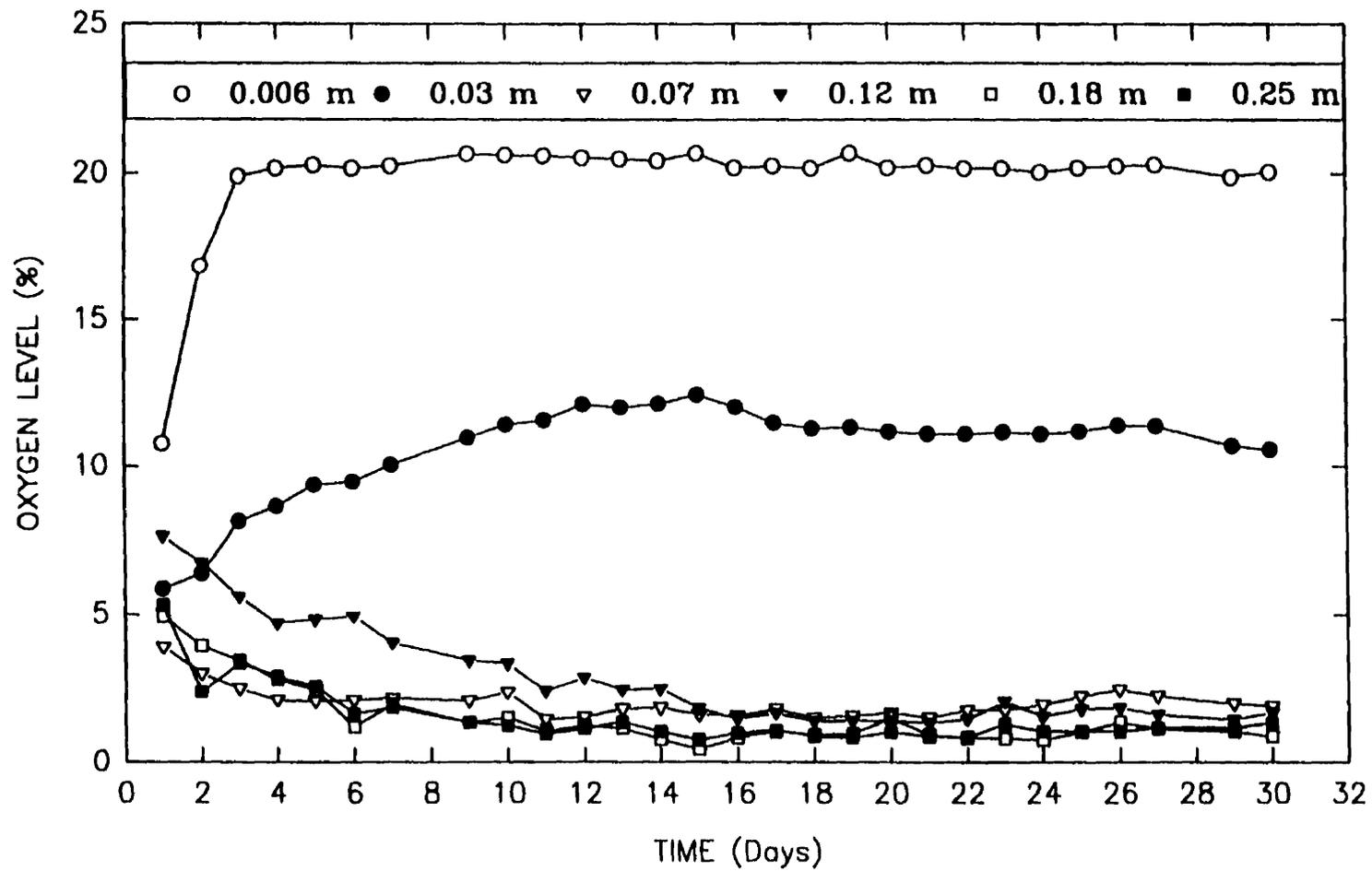
Figure 5.12 Progression of  $O_2$  in Chambers with Channels of Six Varying Lengths and a CSA of  $4 \cdot 10^{-6} \text{ m}^2$
