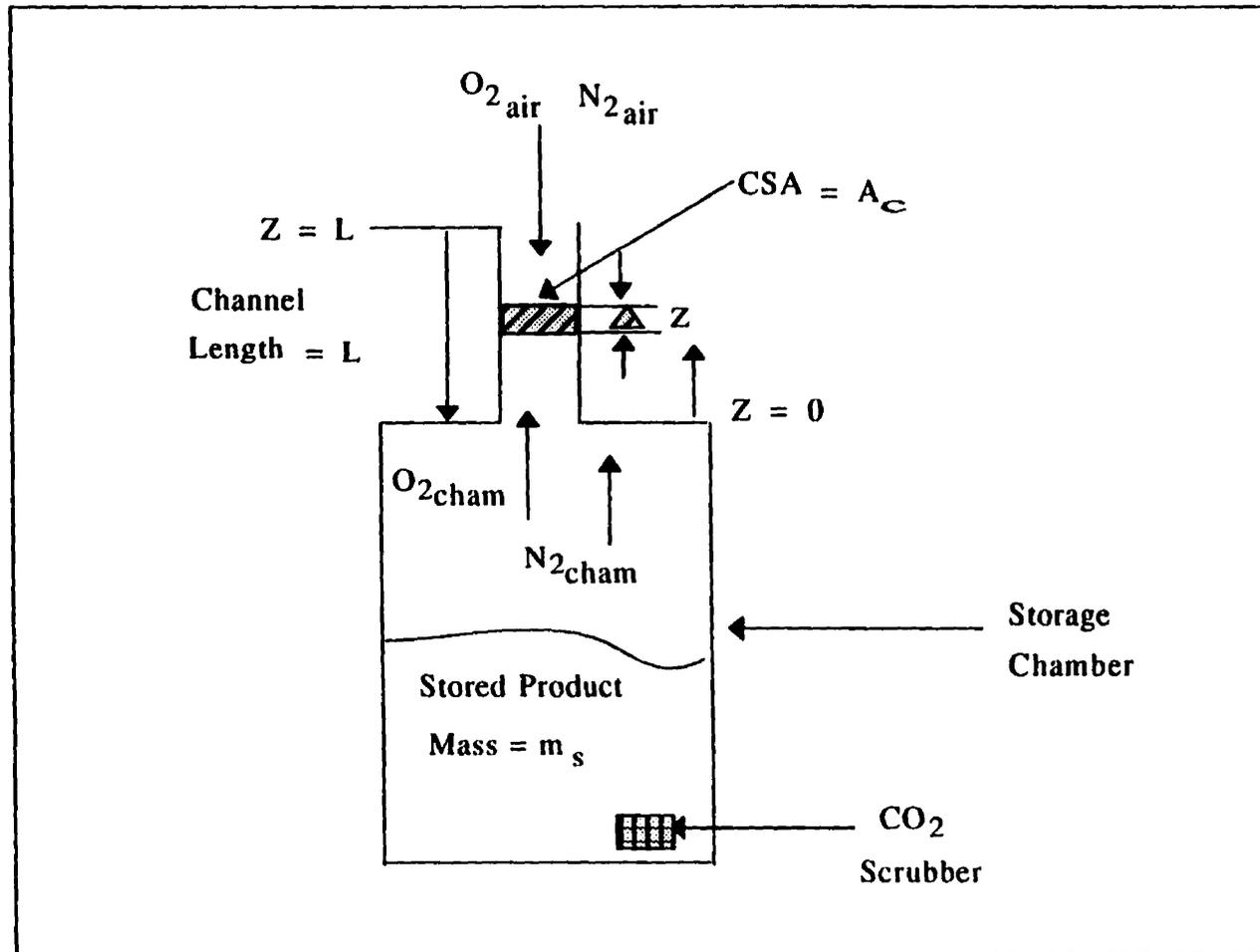
Figure 3.2 Oxygen Diffusion Process into a Storage Chamber Through a Channel
