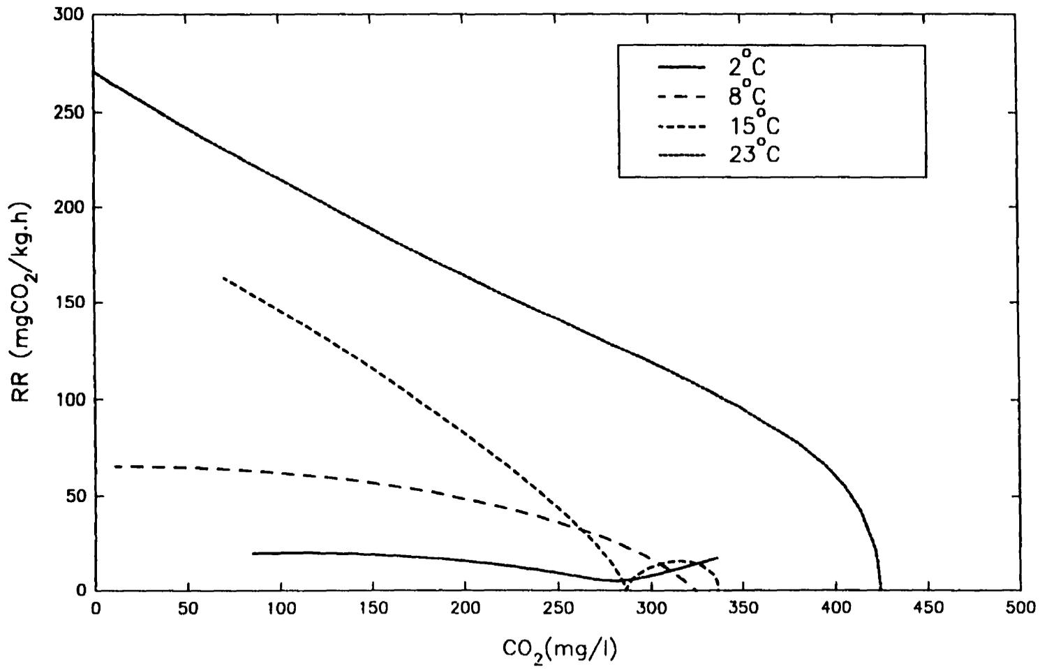
**Figure 5.6** Respiration Rate of Spinach at Four Levels of Temperature as a Function of CO<sub>2</sub> Concentration.
