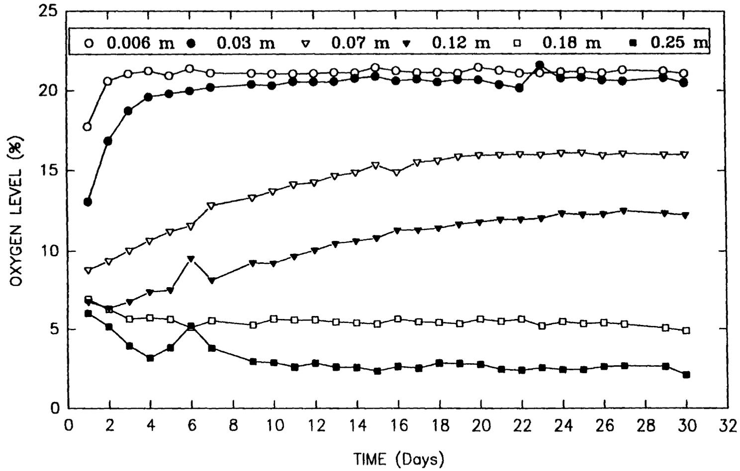
Figure 5.14 Progression of O<sub>2</sub> in Chambers with Channels of Six Varying Lengths and a CSA of 1.15\*10<sup>-4</sup> m<sup>2</sup>
