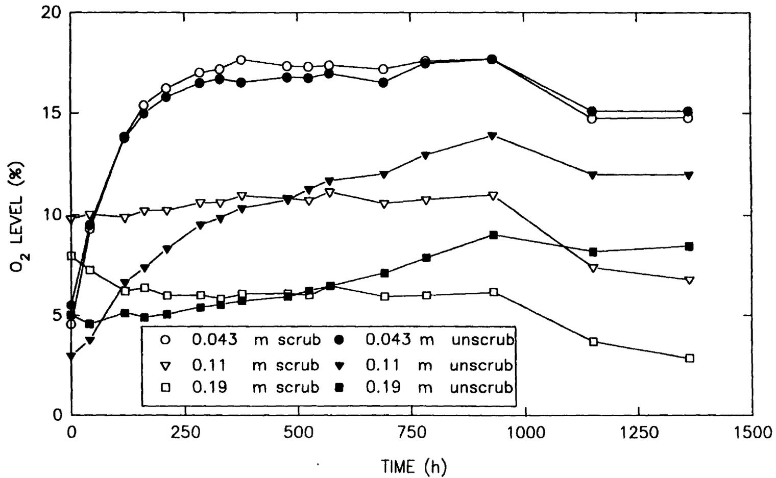
Figure 5.27 Comparison of O<sub>2</sub> Levels in CO<sub>2</sub> Scrubbed and Unscrubbed Chambers for CSA of  $1.7 \cdot 10^{-4} \text{ m}^2$ .
