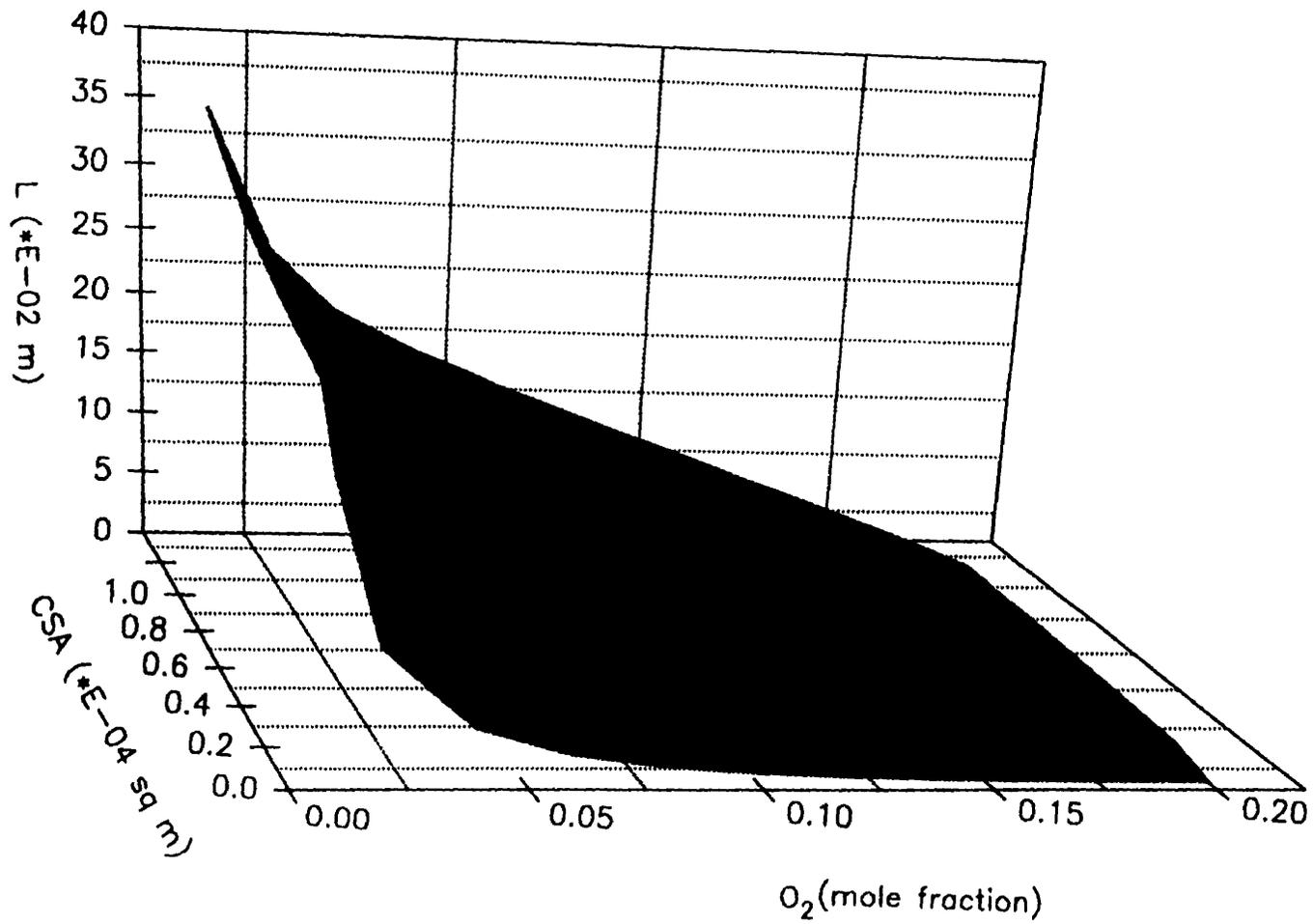
Figure 5.21 The Relationship of Length, Cross Sectional Area of Diffusion Channel and  $O_2$  Steady State Level.
