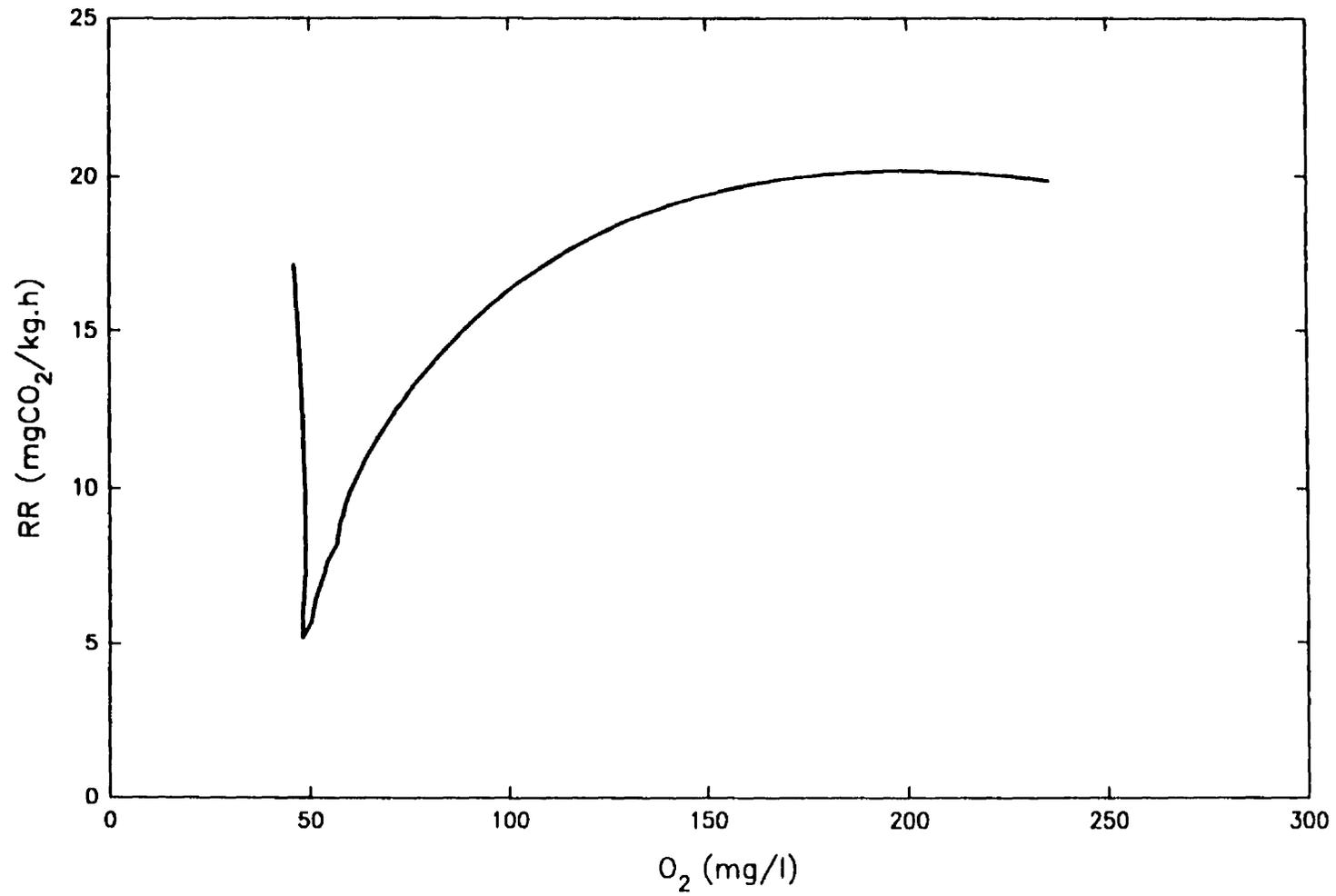
Figure 5.3 Respiration Rate of Spinach at 2°C as a Function of O<sub>2</sub> Concentration.
