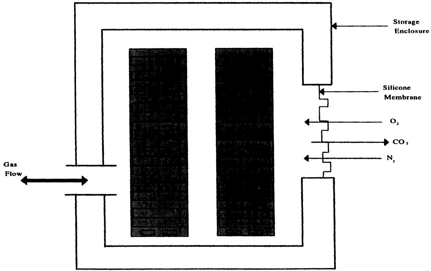
Figure 2.2 Schematic Diagram of a Membrane CA Storage System.
