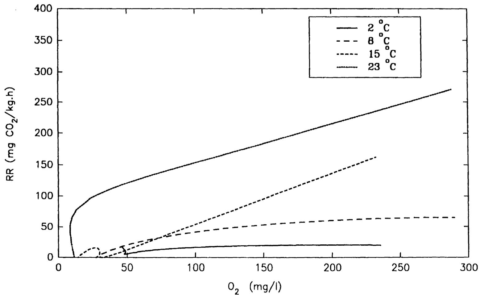
Figure 5.5 Respiration Rate of Spinach at Four Levels of Storage Temperature as a Function of O<sub>2</sub> Concentration.
