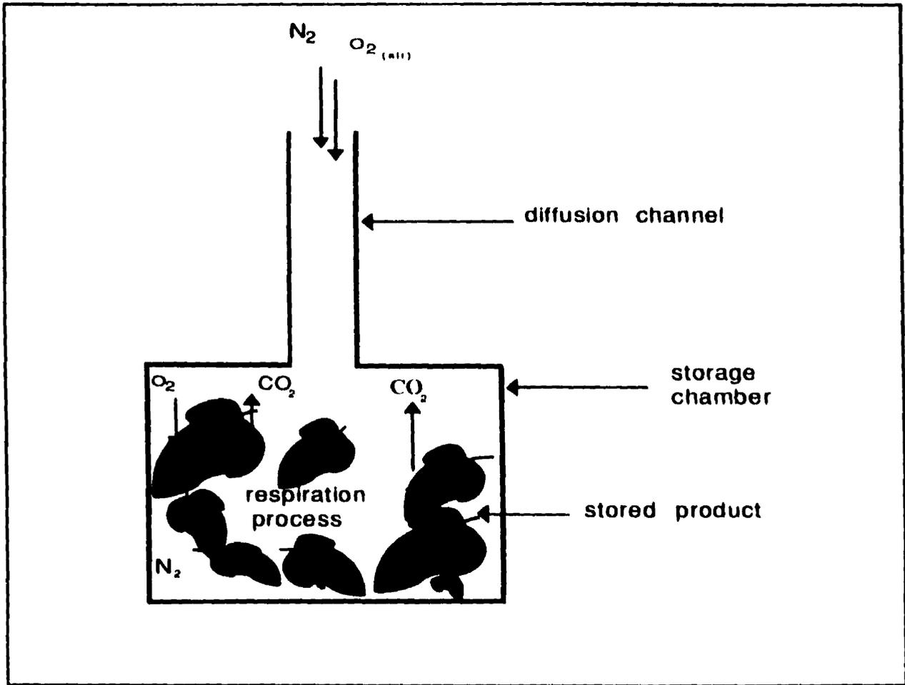
Figure 2.6 Schematic Diagram of The Diffusion Channel System
