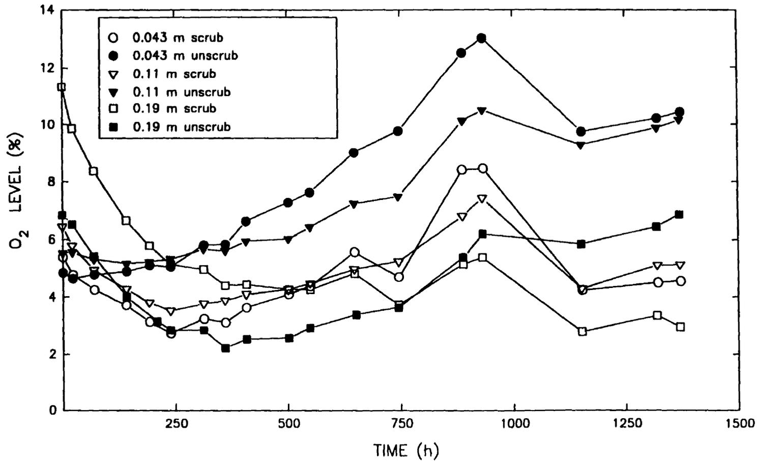
Figure 5.25 Comparison of O<sub>2</sub> Levels in CO<sub>2</sub> Scrubbed and Unscrubbed Chamber for CSA of  $9 \cdot 10^{-6} \text{ m}^2$ .
