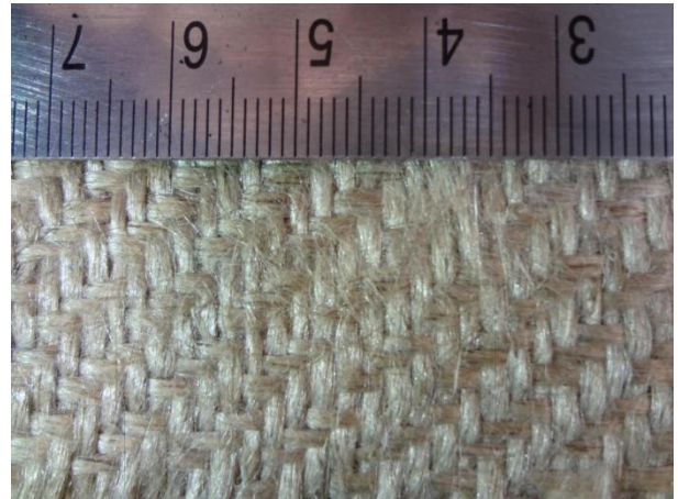
Figure I.2 Left picture: diagram showing a yarn and its parameters. Right picture: image taken by high resolution digital camera to measure the twist angle and yarn diameter
