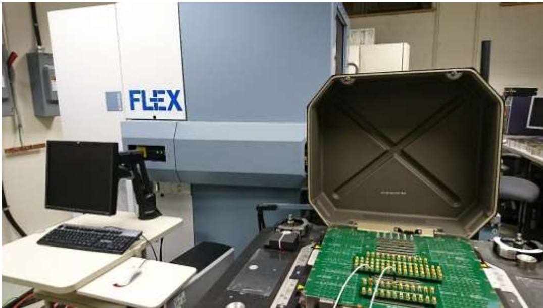
Figure 7.1: Teradyne Flex Tester used for the experimental validation measurement for the coherent subsampling method.
