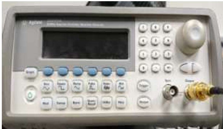
Figure 7.9: Agilent 33220A signal generator with Modulation input.
