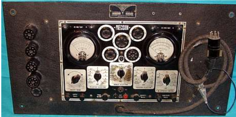
Figure 1.1: Early ATE which can be programmed using knobs and dials.
