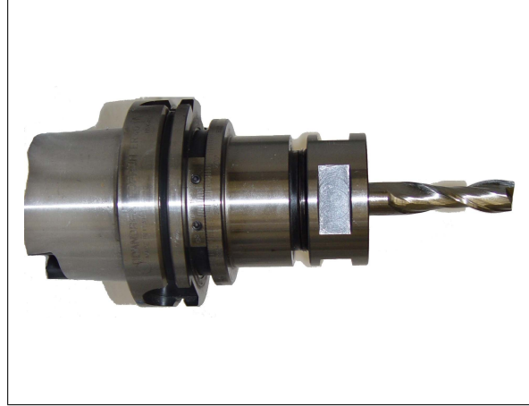
Figure 6.5: Picture of the end-mill mounted on the tool holder
