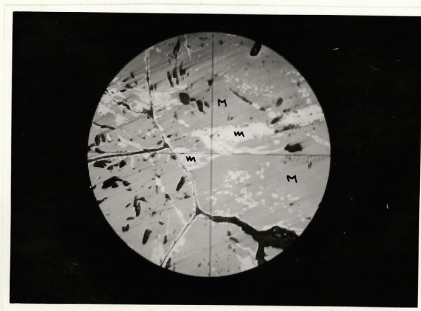
Fig. 19. Photomicrograph showing martitization of magnetite in a zone of brecciation and micro-folding. M-magnetite; m-martite. Reflected light. Medium power. X 84.
