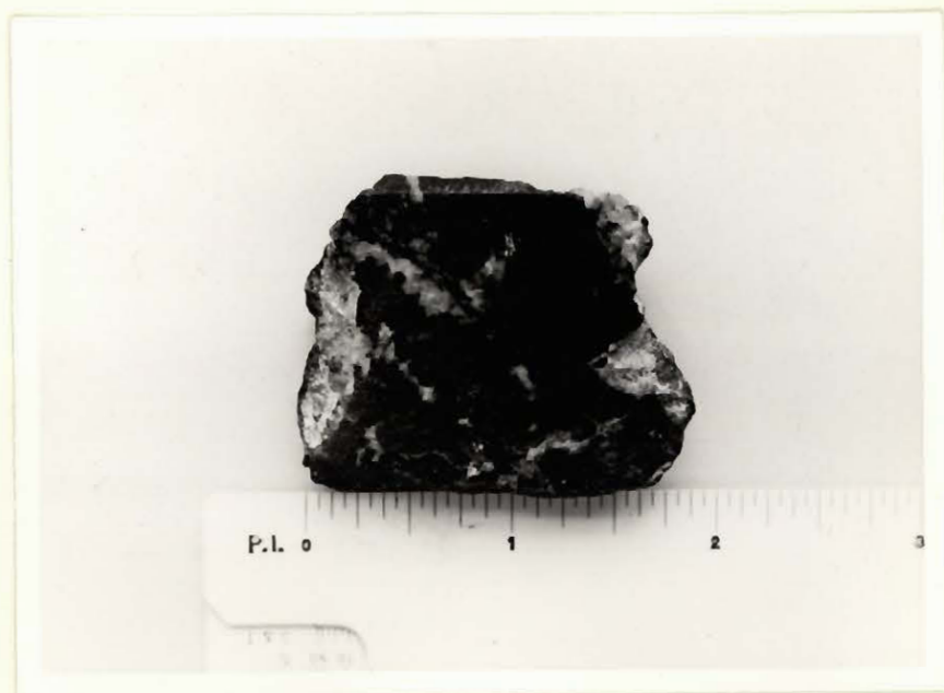
Fig. 41. Photograph of veinlets of dolomite at the contact between serpentinite and enstatite-chlorite rock.
