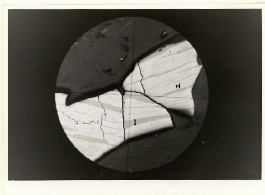
Fig. 39. Photomicrograph of seriate arrangement of ilmenite ex-solution bodies unmixing from hematite. I-ilmenite; H-hematite. Reflected light. Medium power. X 84.
