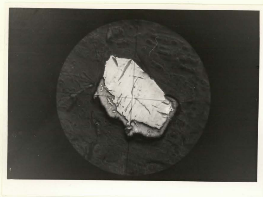
Fig. 35. Photomicrograph showing chalcocite replacing a magnetite grain. Reflected light. Medium power. X 84.
