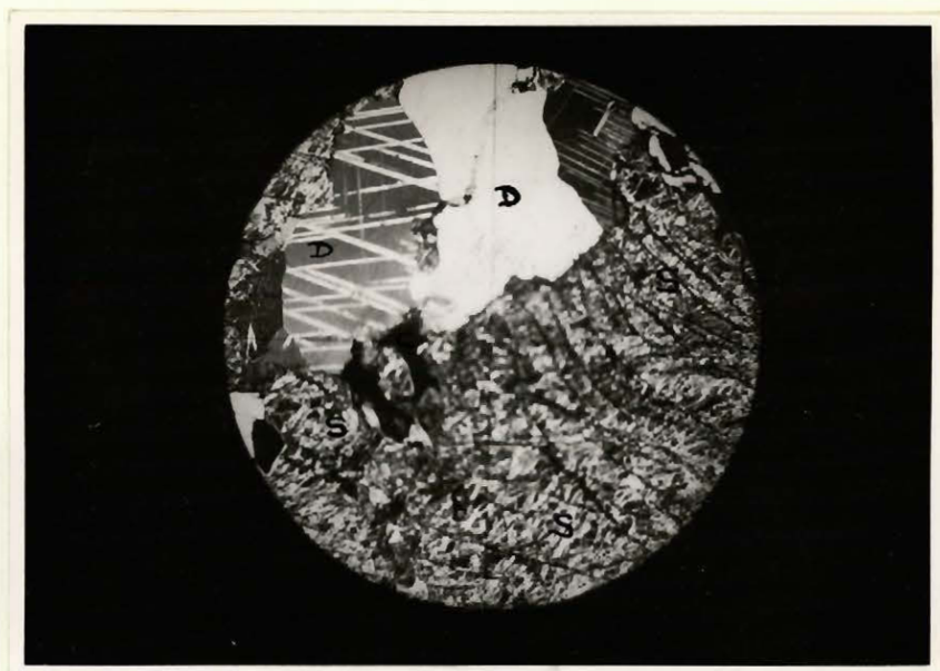
Fig. 23. Photograph of serpentinite altered to serpophite. D-dolomite; C-chalcocite; S-serpophite. Cross nicols. Medium power. X 29.
