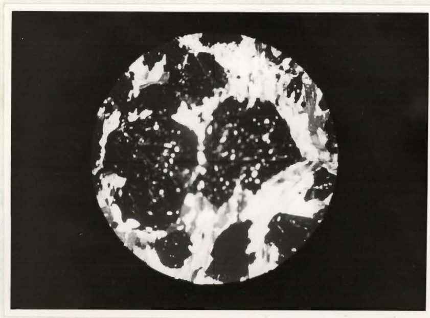
Fig. 6. Photomicrograph of poikiloblastic garnets in feldspar-hornblende-biotite gneiss. Cross nicols. Low power X 9.
