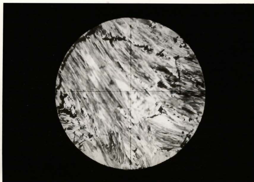
Fig. 15. Photomicrograph showing a mass of fibrous grunerite of the iron silicate formation. Cross nicol. Medium power. X 29.
