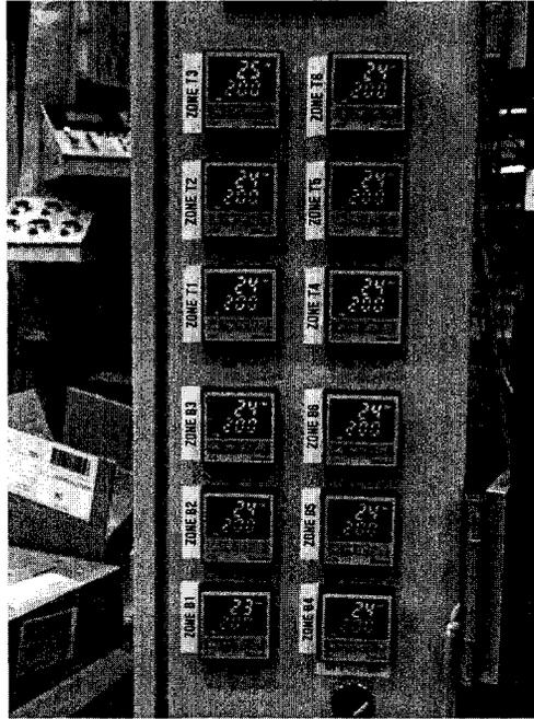
Figure 4-5: PID control panel (for all 12 heater zones)
