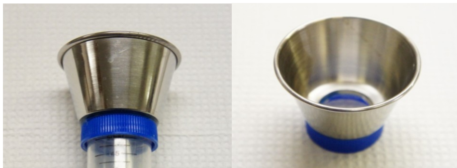
Figure 10: The spill- and evaporation-proof cap used to prevent solvent evaporation from the extraction tube during the PUASE process
