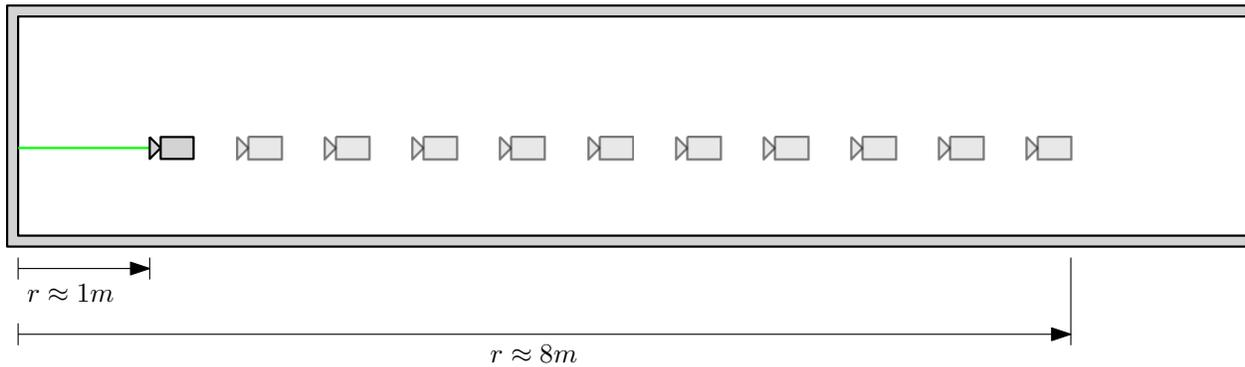
Figure 3.3: Test setup for range variance vs. distance.
