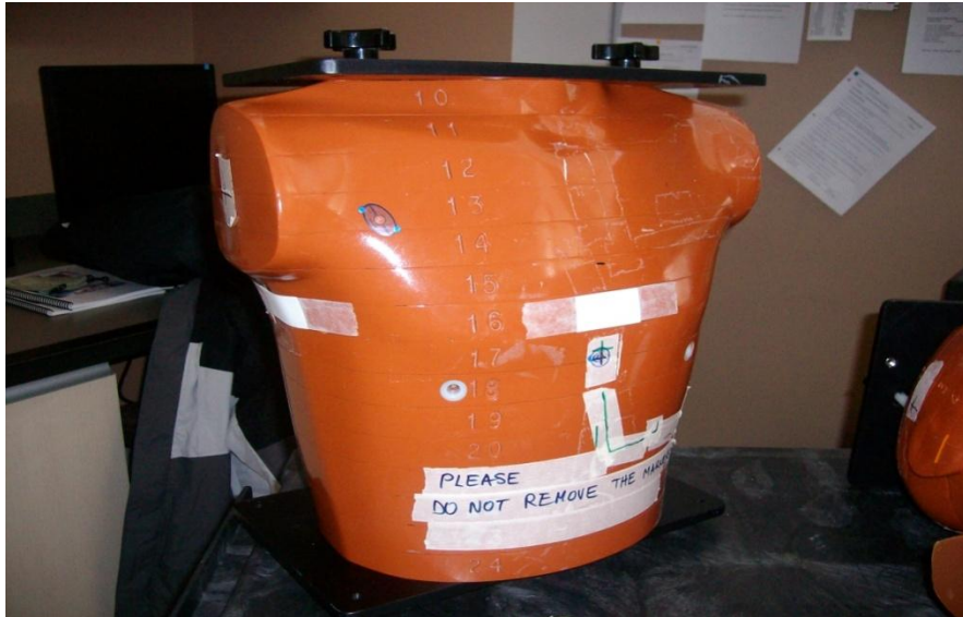
Figure 3.12: Thorax region of Rando phantom with skin dose films taped to the surface.
