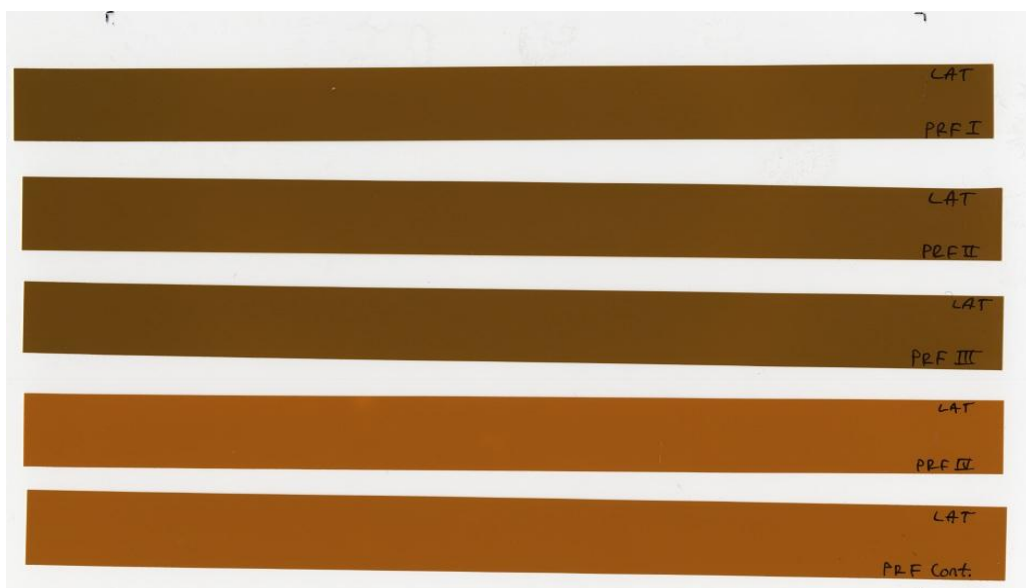
Figure 3.13: XR-QA film strips used to measure lateral dose profiles in the pelvic region. The irradiated films are noticeably darker.
