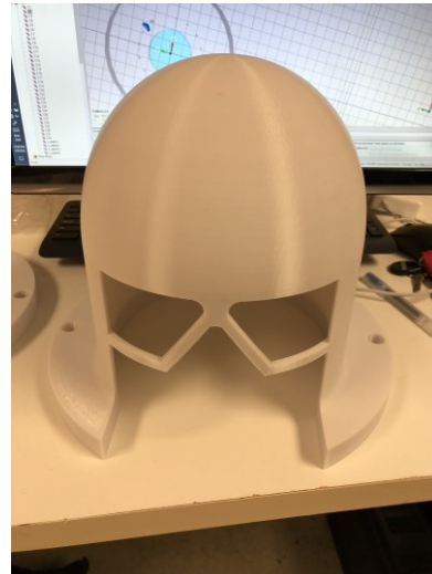
Figure 38: a) 3D CAD model of head shaped housing. b) 3D printed housing: vertical rods and top support piece not shown.
