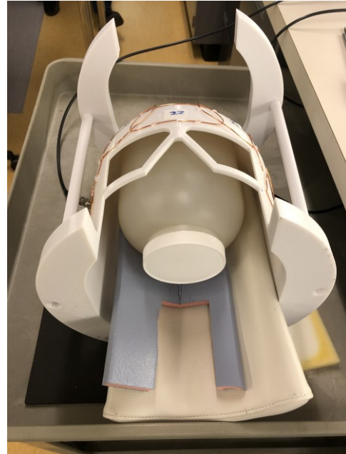
Figure 42: a) Attaching receive elements to housing and geometrically decoupling with all adjacent loops b) ^{31}\text{P} phantom placement inside the housing
