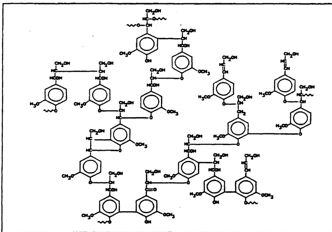
Figure 1.6. Depiction of a hypothetical fragment of a softwood lignin molecule in two of its three dimensions.
