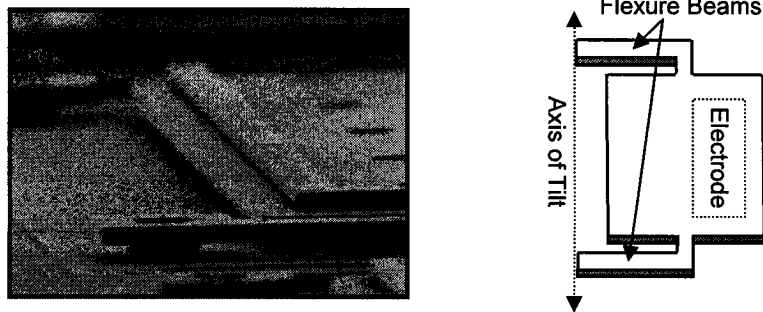
Figure 4.3: SEM and Geometry of Electro_1 Micromirror
