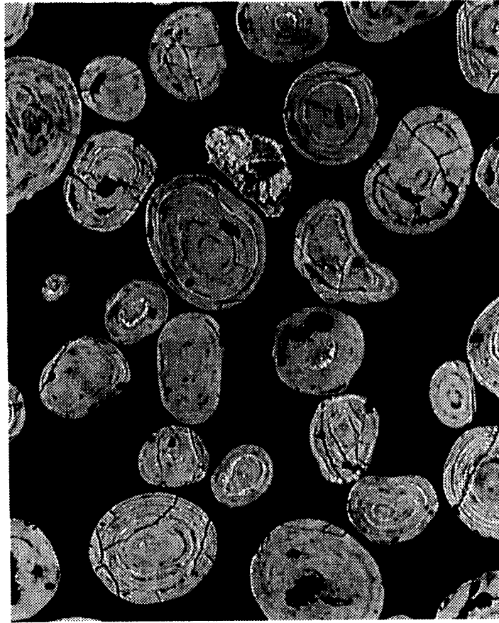
Figure 12: Cross-sectional view of the oxides produced in a fluid bed reactor that illustrates the onion-skin structure (low magnification). [1]
