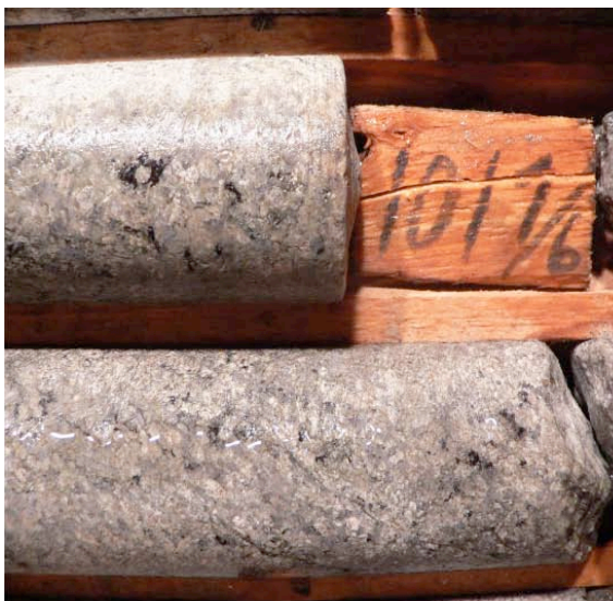
Figure 4.1 Photographs of core sections from the West Clearwater impact structure. A) Pink medium-grained biotite-hornblende granite from a depth of ~310 m in drill hole 3-63. B) Medium- to coarse-grained hornblende-biotite gabbro (375 m, drill hole 1-63). C) Fine-grained gray biotite tonalite cut by veins of pseudotachylite (~30 m, drill hole 3-63). D) Fragmental breccia matrix (~50 m, drill hole 4-63).
