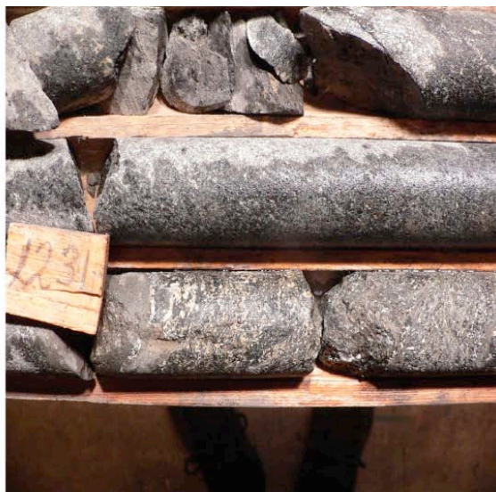
Figure 4.1 Photographs of core sections from the West Clearwater impact structure. A) Pink medium-grained biotite-hornblende granite from a depth of ~310 m in drill hole 3-63. B) Medium- to coarse-grained hornblende-biotite gabbro (375 m, drill hole 1-63). C) Fine-grained gray biotite tonalite cut by veins of pseudotachylite (~30 m, drill hole 3-63). D) Fragmental breccia matrix (~50 m, drill hole 4-63).
