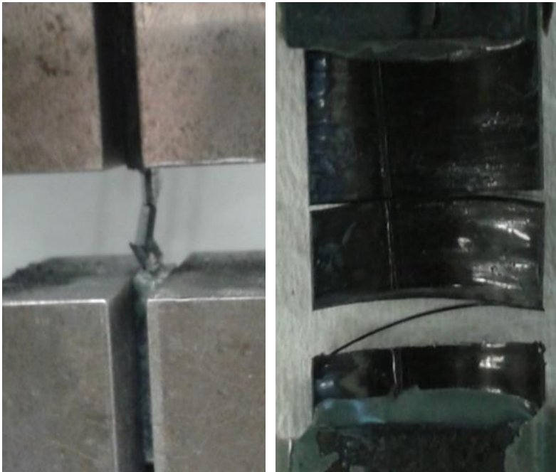
Figure 34 - Typical Failure of Unidirectional [90] Carbon Fiber
