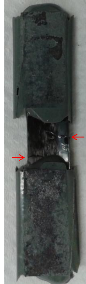
Figure 35 - Typical Failure of Unidirectional [0] Carbon Fiber
