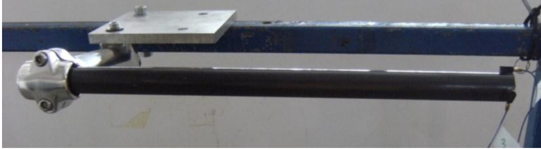
Figure 49 - Impact Hammer Clamped Test Set-Up
