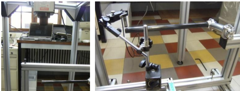
Figure 52 - IET Clamped Test Set-Up Left: Laser; Right: Microphone
