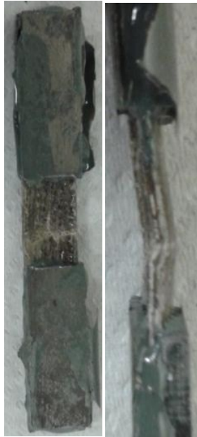
Figure 41 - Failure Mode of [0] ampliTex Light Unidirectional Flax Fiber Left: Inner surface of failed specimen Right: Detailed side view of failure location
