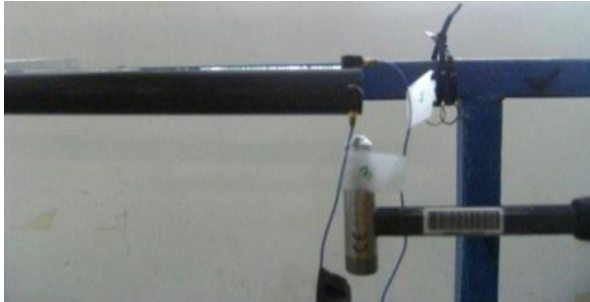
Figure 50 - Location of Impact for Clamped Boundary Condition
