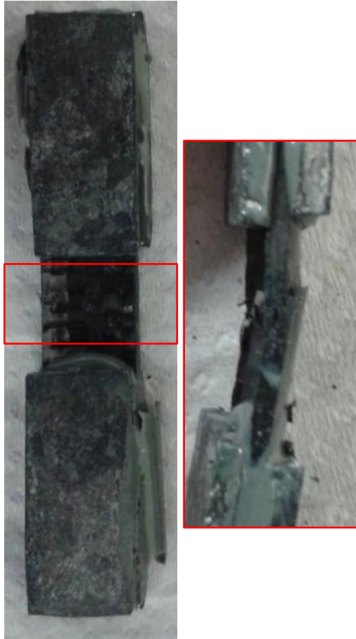
Figure 36 - Typical Failure of Plain Weave Carbon Fiber
