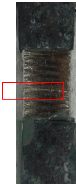
Figure 44 - Failure Mode of [90] ampliTex Standard Unidirectional Flax Fiber Inner surface of failed specimen. Red box indicates location of failure.
