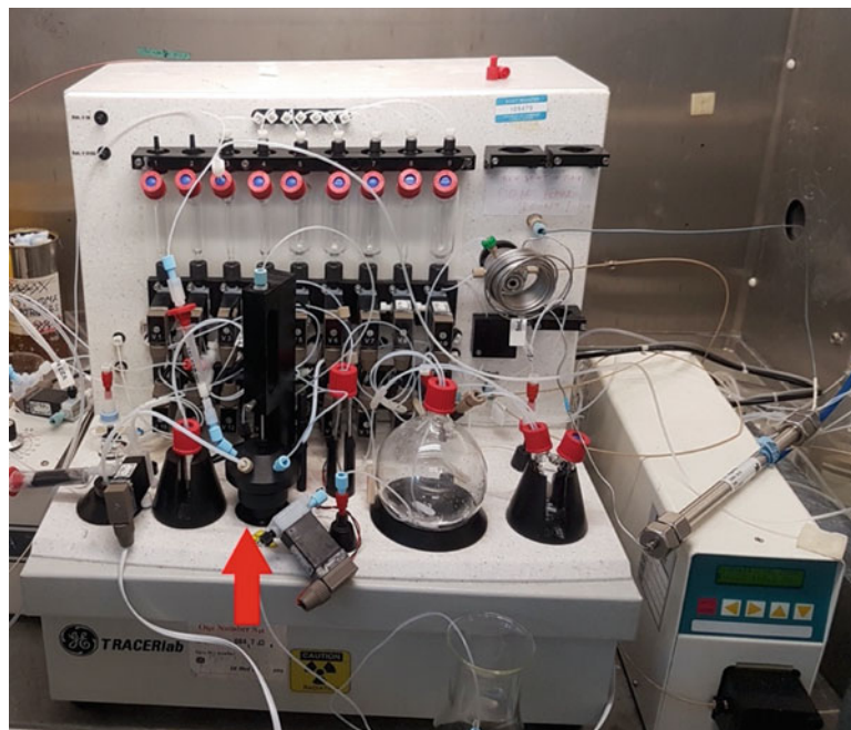
Fig. 3 GE TRACERlab FX FN automated synthesizer. Reactor is arrowed (red arrow)
