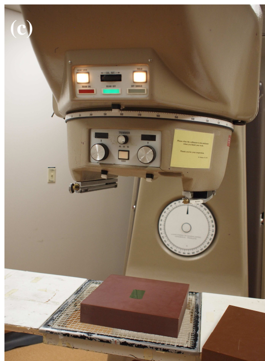
Fig.7. Film Irradiations at ^{60}\text{Co} using a Theratron 780 cobalt unit. (a) Schematic diagram of ^{60}\text{Co} irradiation. (b) Picture of film irradiation setup. (c) The film is placed at a depth of 5 cm in a solid water phantom.
