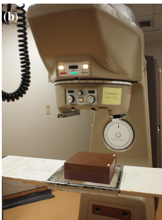
Fig.7. Film Irradiations at ^{60}\text{Co} using a Theratron 780 cobalt unit. (a) Schematic diagram of ^{60}\text{Co} irradiation. (b) Picture of film irradiation setup. (c) The film is placed at a depth of 5 cm in a solid water phantom.
