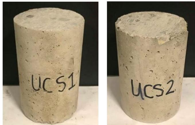
Figure 3-6: UCS concrete Samples
