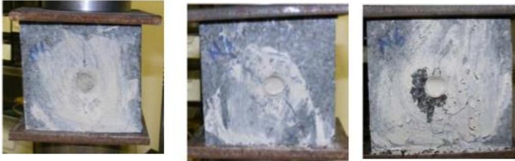
Figure 2-18: Expansive cement under uniaxial loading (Mitri & Musunuri,2009)
