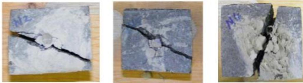
Figure 2-19. Expansive cement under free load (Mitri & Musunuri, 2009)
