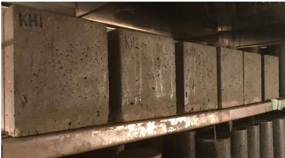
Figure 3-4: Curing of concrete cubes in humidity room
