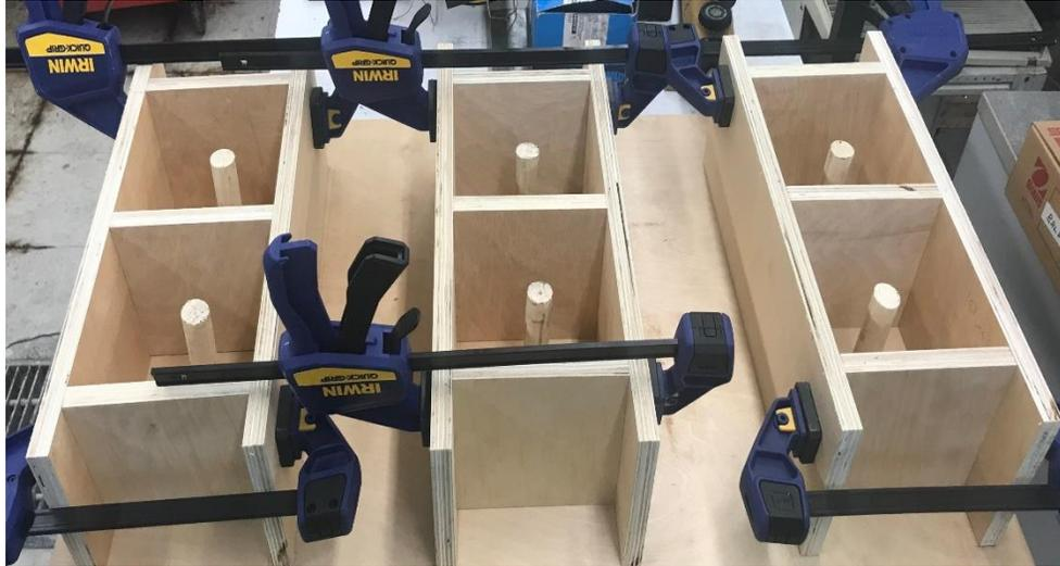
Figure 3-3: Concrete molds
