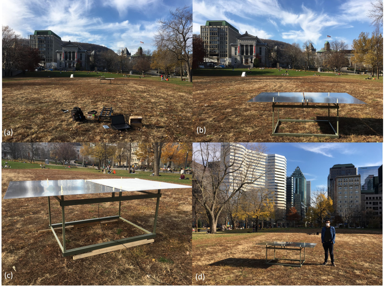
Figure 3.20: (a), the site where we took the measurements, with the materials used: toolbox, VNAs, and other tools; (b) the antenna in East-West orientation; (c) the antenna with added height (of approximately 8 cm), and one flipped panel; (d) antenna compared to myself in terms of size.
