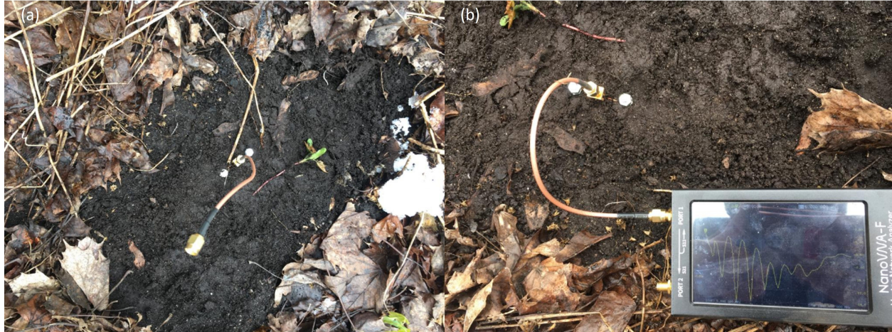
Figure 4.7: (a) Threaded rods placed entirely inside soil, before being connected to the VNA. (b) Threaded rods placed entirely inside soil, connected to the VNA.
