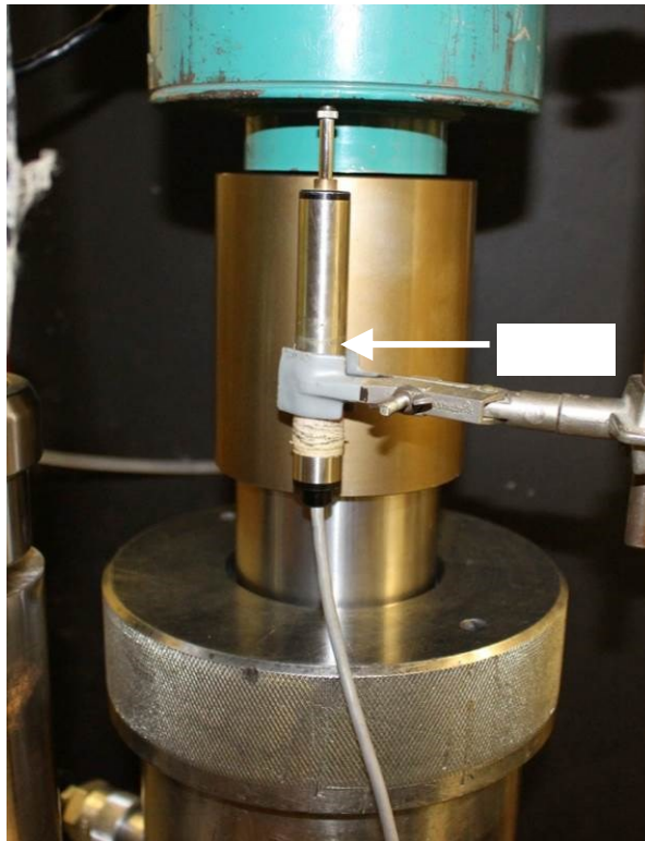
Fig. 15: The LVDT, measures displacement of the piston
