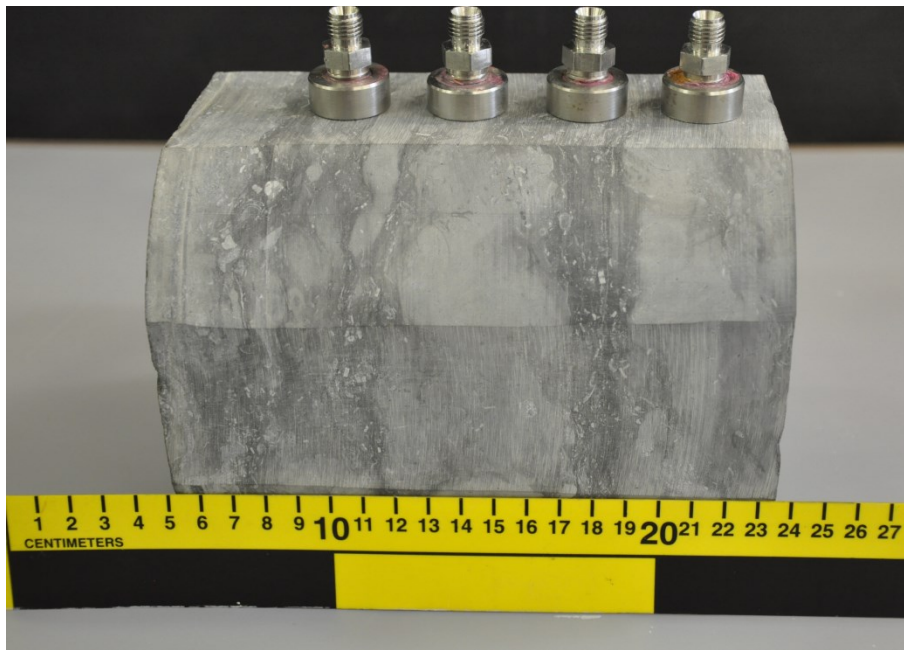
Figure 2.4: Photograph of the Cobourg Limestone surface presenting the typical visually heterogeneous matrix phases.
