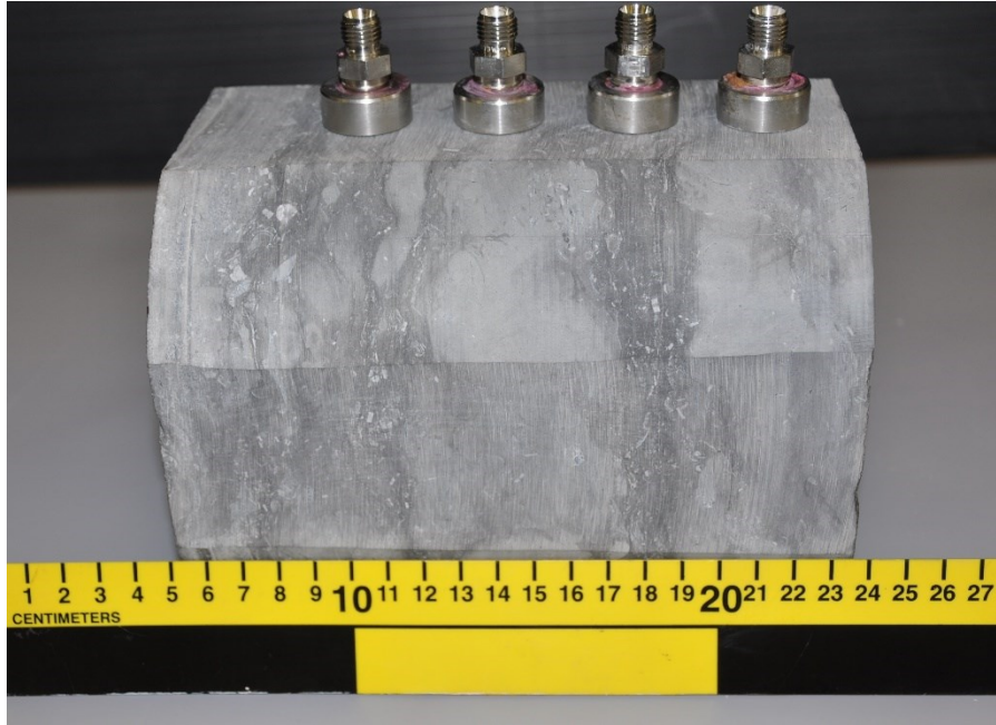
Figure 6.1: Sample of Cobourg Limestone with cut flat surfaces and entry port connectors positioned on the specific phases.
