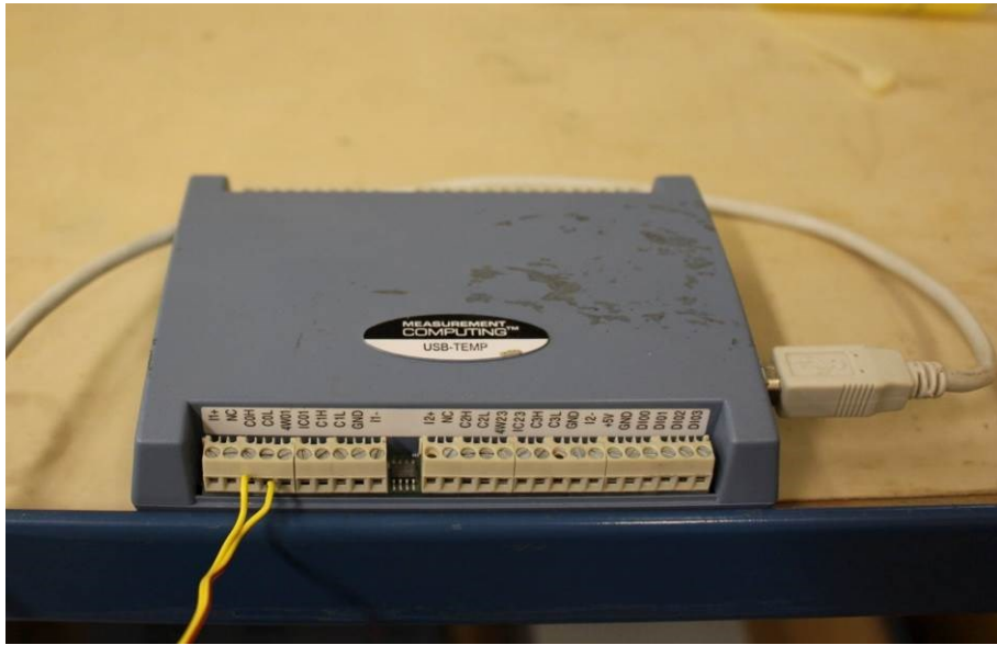
Fig. 14. The DAQ system, USB-TEMP, connected to thermocouple Type K
