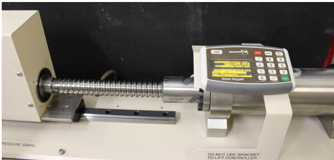
Fig 11: GDS Controller #1, which controls the axial load
