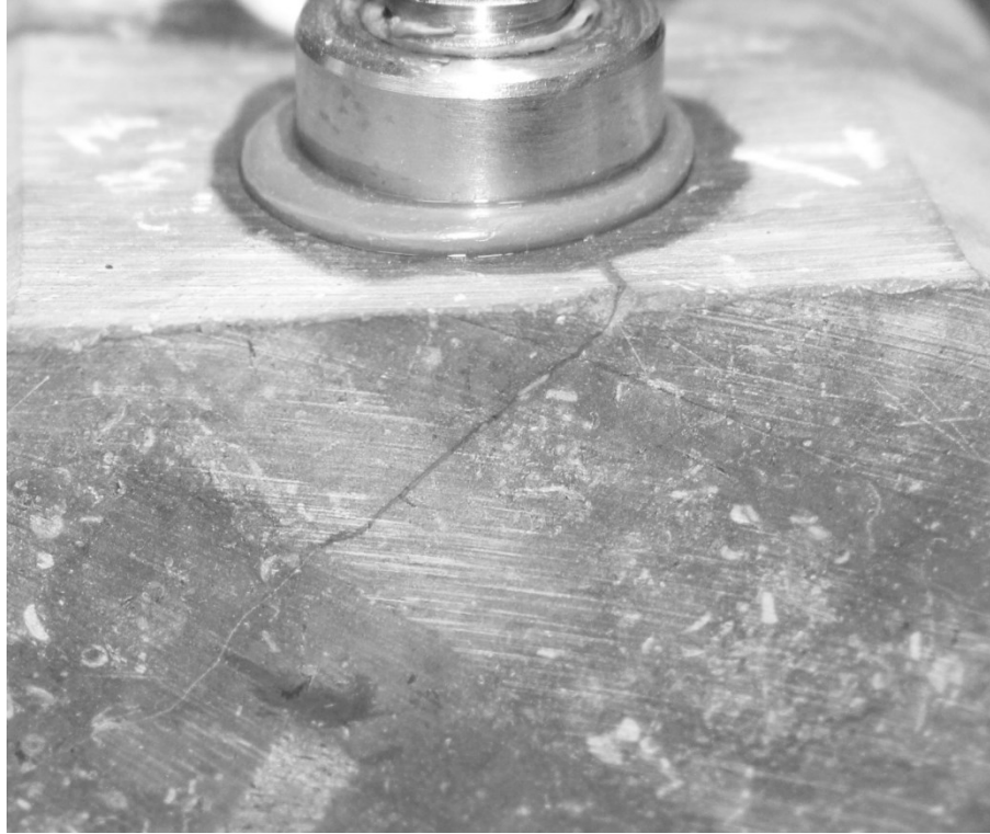
Figure 6.25: Close up view of the Location 1 on the Cobourg Limestone; the crack that had formed near the entry port connector was accentuated, for visual appreciation, by wetting the surface with water.
