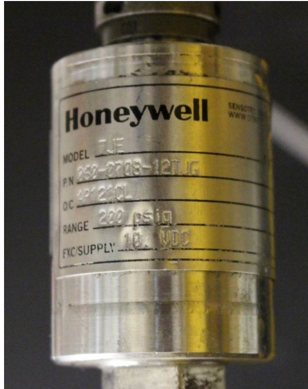
Fig. 16: A Close-up of Pressure Transducer
