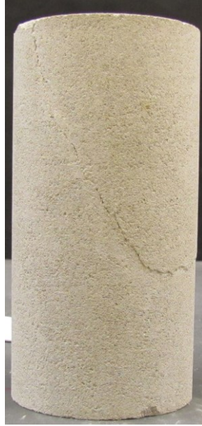
Figure 7.4: Indiana Limestone post failure subjected to confining stress of 15 MPa.
