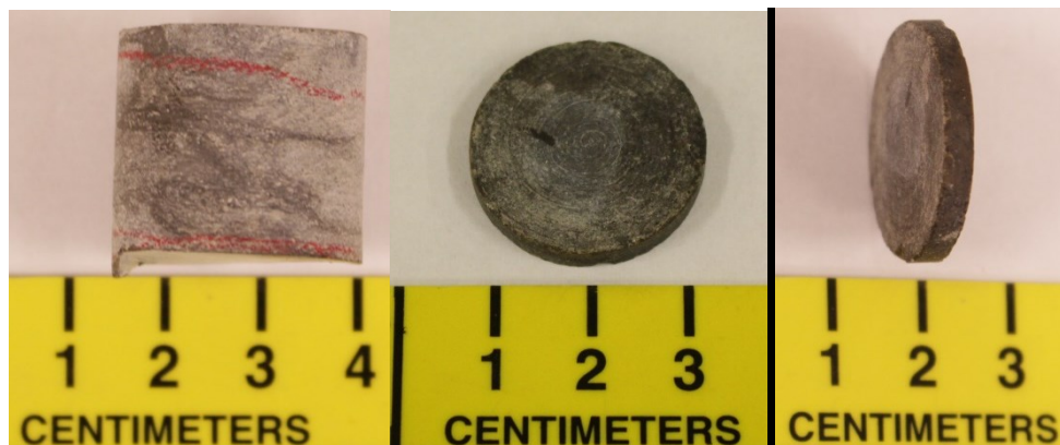
Figure 1: Disk preparation and final sample
