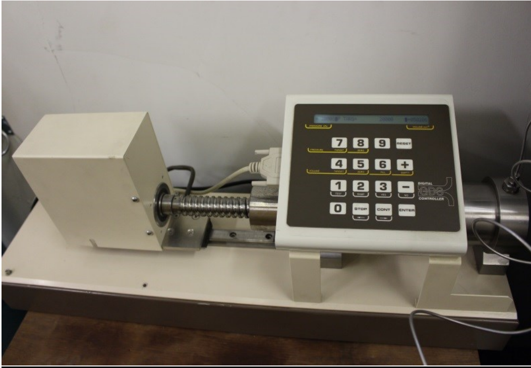
Fig. 12: GDS Controller #2, which controls the radial pressure inside the Obert-Hoek Cell
