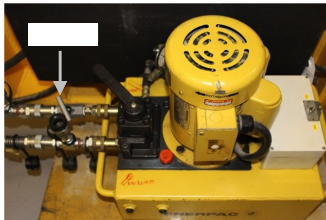
Fig 4: Electric Hydraulic Pump used for large piston movements
