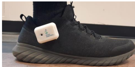
Figure 1. Heel2Toe Sensor Attached to the Shoe
