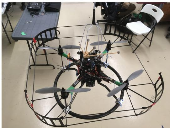
FIGURE 5.1: Modified AscTec Pelican used for Flight Testing
