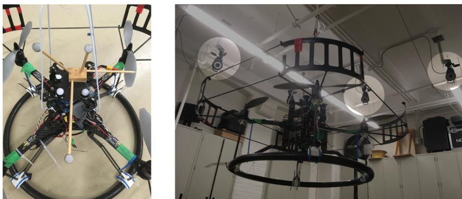
FIGURE 5.2: VICON Motion Capture Flight Test Setup
