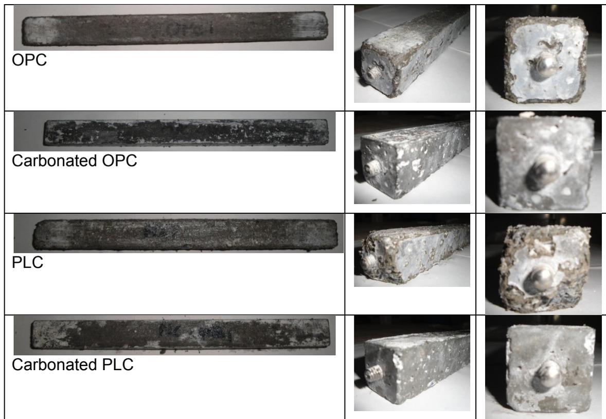
**Figure 4-9: Mortar bars following 10 months of exposure to  $MgSO_4$  at  $5^\circ C$**
