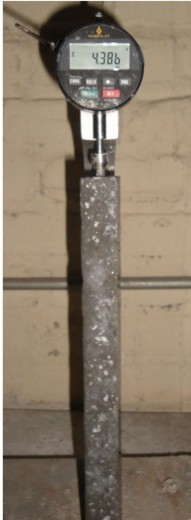
**Figure 3-5: Change in length of mortar bar measurements**
