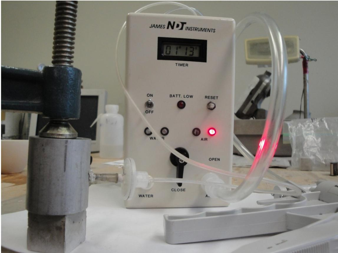
**Figure 3-7: Surface air permeability test setup**
