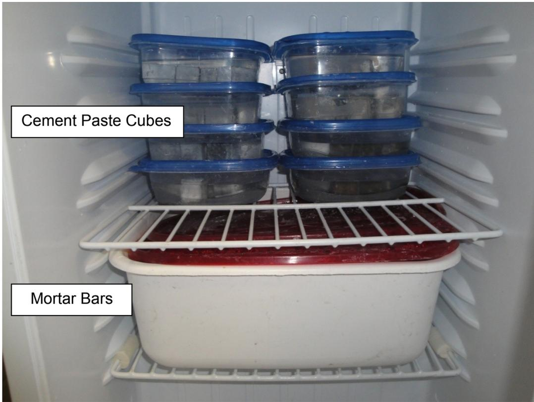
**Figure 3-2: Low temperature sulphate attack test setup**
