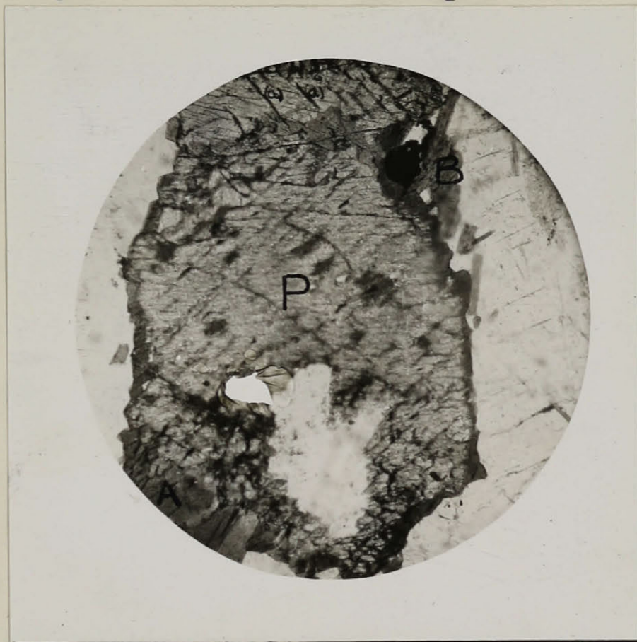
Fig. 4. Pyroxene (P), with a reaction rim of amphibole (A). (B)-biotite. (a)- amphibole. X14
